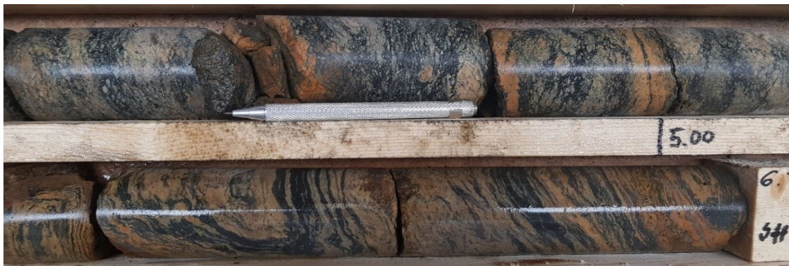
Fig. 16. Drill core showing porphyritic volcaniclastic sedimentation features in the top row, with felsic clasts in a mafic matrix. In the bottom row, strongly banded, deformed tuffite with bands of mafic/intermediate and felsic composition. Drill core 18MUS002, depth 5m.
