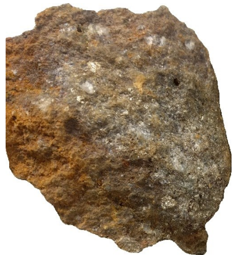
Fig. 78. Grab sample of a relatively tourmaline poor, moderately oxidized quartz-tourmaline-pyrite vein grading 14.75 ppm Au (sample MJ-34). Sample width is approx. 15 cm.
