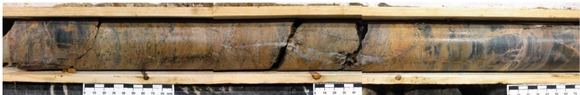
Fig. 55. Drill core showing a cross cutting quartz-albite vein albitizing the siliciclastic host rock. Drill core MJ-5, depth 45 m.
