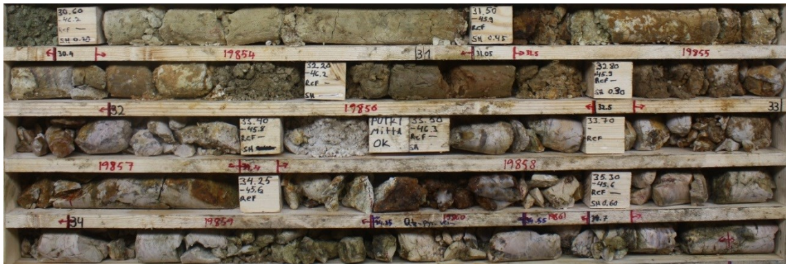
Fig. 101. Drill core showing strongly kaolinized and oxidized mineralized zone. Intense kaolinization causes strong core loss. At 34.35 m is a 0.3-m-wide quartz-pyrite vein that grades 11.6 ppm Au. Drill core 18MUS105, depth 30-37 m.
