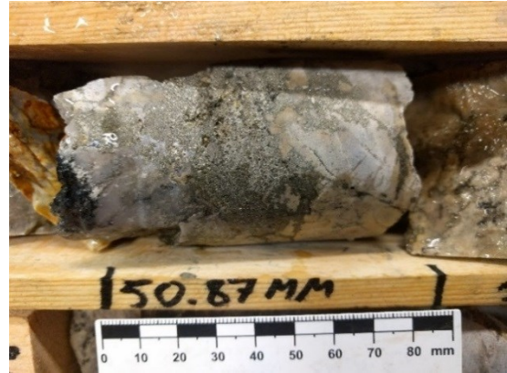
Fig. 72. Drill core showing a massive pyrite vein with only little quartz, yielding a gold value of 0.37 ppm Au. Drill core MJ-9, depth 50.9 m.
