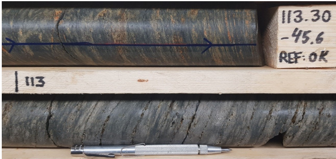
Fig. 66. Drill core showing a weakly altered and veined intermediate tuffite (top row) being affected by strong sericitization (bottom row). Original albite- and carbonate-bearing veins have been mostly weathered away in the sericitized part. Drill core 18MUS013, depth 113 m.
