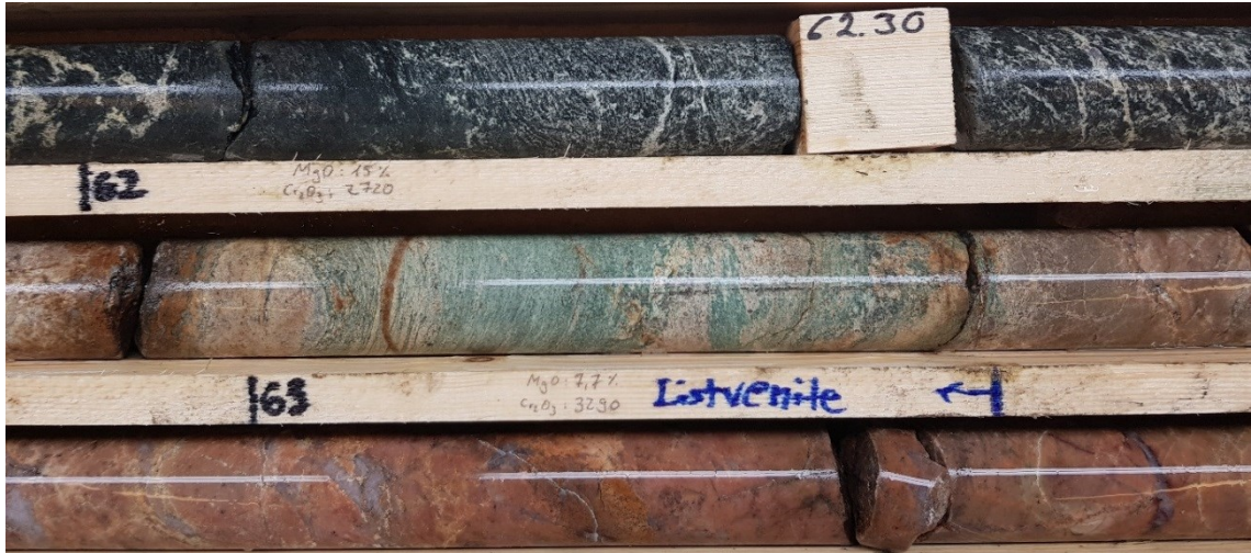
Fig. 53. Drill core showing ultramafic tuff (top row) in contact with albitized and silicified siliciclastic metasediments (bottom row). In the contact zone between the rock units occurs listvenite as a totally carbonate altered ultramafic tuff (middle row). Drill core 18MUS001, depth 63 m.
