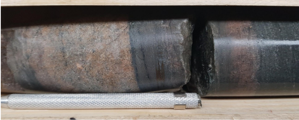
Fig. 17. Drill core showing a ~5 cm thick arkose quartzite interlayer in an intermediate tuffite. Drill core 18MUS013, depth 168 m.
