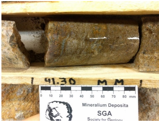
Fig. 60. Drill core showing a laminated ankerite-dolomite vein with quartz clasts which give the vein a conglomeratic appearance. A small late stage calcite vein is cutting the vein perpendicularly. Drill core MJ-9, depth 41.3 m.
