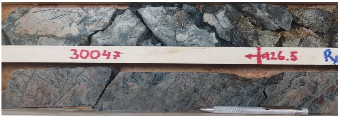
Fig. 65. Drill core showing biotitization. Both rows show gold mineralized intermediate tuffite that is strongly enriched with biotite, which occurs as biotite stringers (e.g. top row on the left) and disseminated in the host rock matrix that is distinguishable as dark spots in a bleached matrix (e.g. bottom row on the left). Drill core 18MJ010, depth 126.5 m.
