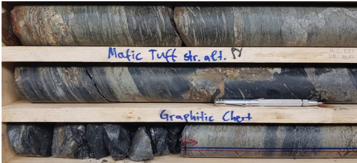
Fig. 48. Drill core showing interbedded mafic tuff and graphitic chert. The mafic tuff in the top row shows albite and quartz veins in a mafic matrix and is most likely a zone of strong deformation. The unit is strongly veined with pyrite rich quartz-albite-(carbonate) veins, that are commonly oxidized. The bottom row comprises abundant graphite that is broken up, unlike the rest of the core. Drill core 18MUS013, depth 45 m.
