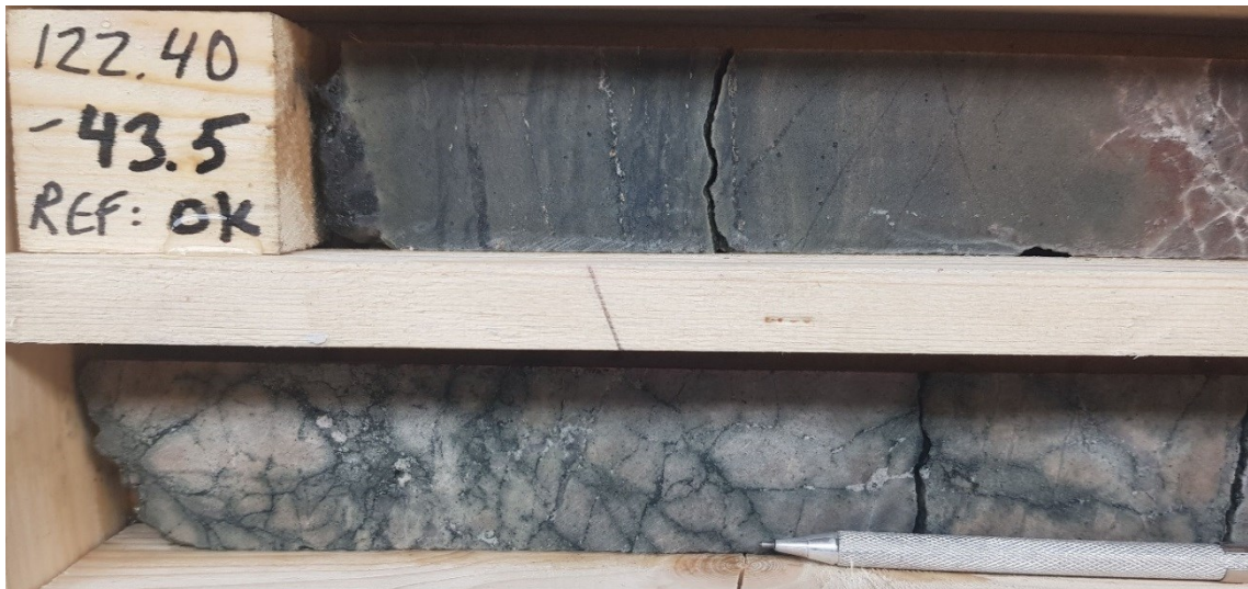
Fig. 64. Drill core showing biotitization. The top row shows relatively unaltered intermediate tuffite outside of the proximal alteration zone. The bottom row shows the onset of the proximal alteration zone with strong biotitization. The rock appears bleached and shows intense biotite stringers. Drill core 18MJ010, depth 122.4 m.
