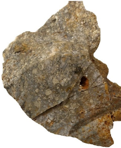
Fig. 75. Grab sample of a relatively unoxidized quartz-tourmaline-pyrite vein grading 10.95 ppm Au (sample MJ-35). Sample width is approx. 15 cm.
