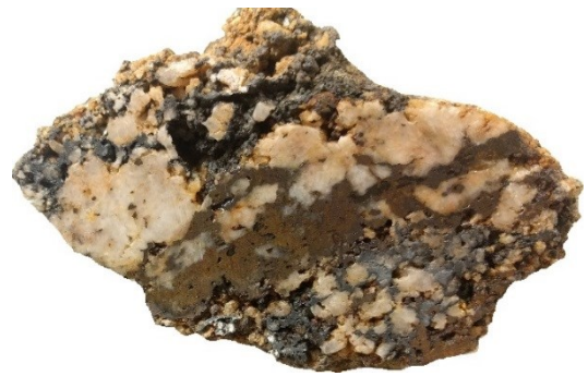
Fig. 100. Grab sample of a Mn weathering crust (blueish-grey) (sample MJ-25). The Mn crust is located on the outer, vuggy parts of a quartz-pyrite vein. The center of the sample is oxidized pyrite (brown). The sample is grading 13.1 ppm Au. Sample width is approx. 15 cm.
