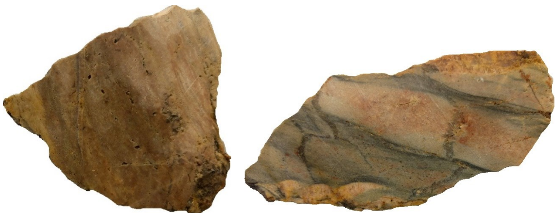
Fig. 18. Arkose quartzite grab samples. (Left) Grab sample MJ-22 from the Mustajärvi artisanal pit. Albitized arkose quartzite without substantial amounts of mica. (Right) Grab sample MJ-37 from the Mustajärvi study area. Banded
