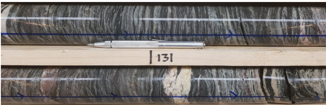
Fig. 47. Drill core showing a strongly banded mafic tuff layer. Perhaps a zone of strong deformation. Drill core 18MUS013, depth 131 m.
