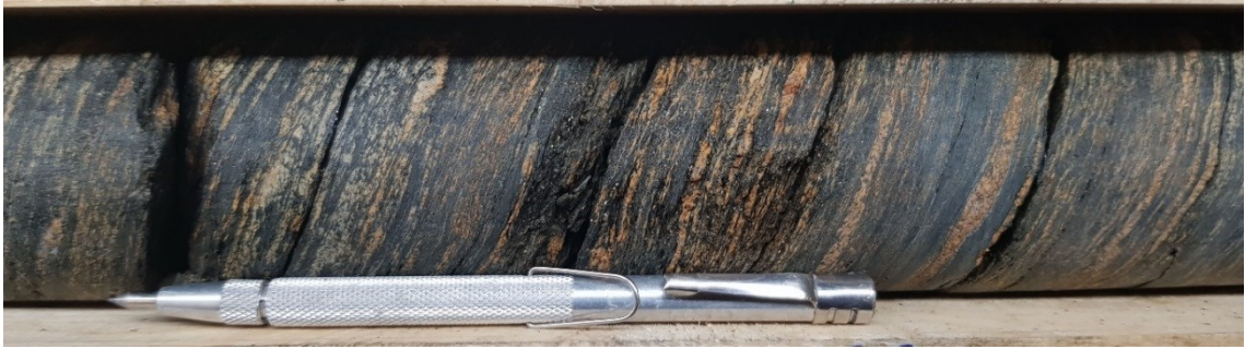
Fig. 31. Drill core showing ultramafic tuff with a strong schistosity and intensive parallel quartz-albite-carbonate veining. Drill core 18MUS013, depth 12 m.
