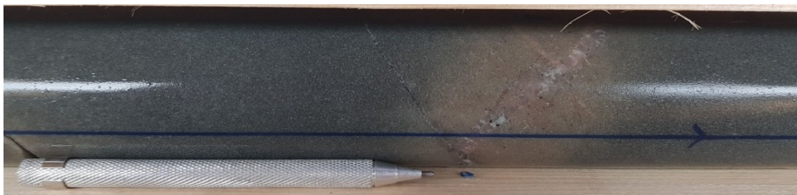
Fig. 50. Drill core showing a quartz-albite vein with a distinct albitization halo in the least altered intermediate tuffites. Drill core 18MUS014, depth 127 m.
