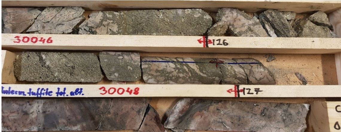
Fig. 79. Drill core showing a two-meter-thick drill intercept of high-grade pyrite mineralization (2 m at 45.1 ppm Au). The mineralization comprises only marginal amounts of tourmaline and quartz. Tourmaline occurs as small bands in pyrite. Drill core MJ010, depth 126 m.
