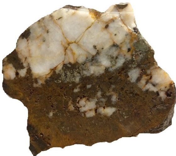
Fig. 77. Grab sample of a tourmaline poor, quartz rich, strongly oxidized quartz-tourmaline-pyrite vein grading 63.8 ppm Au (sample MJ-27). Sample width is approx. 15 cm.
