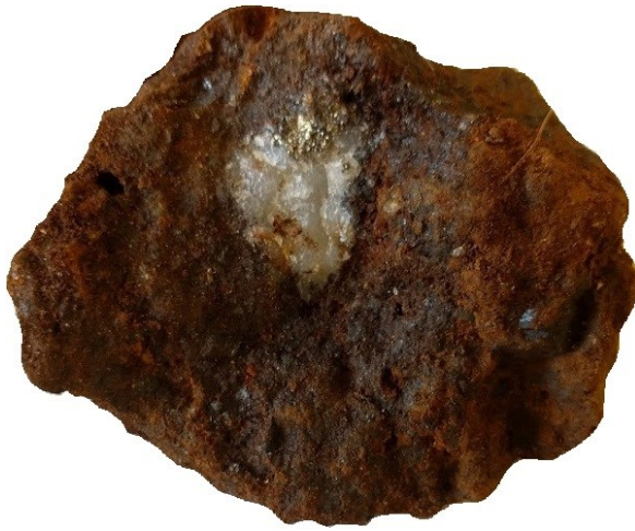
Fig. 99. Grab sample of a heavily oxidized quartz-tourmaline-pyrite vein grading 79.8 ppm Au (sample Mus-3). Only a large quartz clast and some relict pyrite are recognizable. Sample width is approx. 15 cm.
