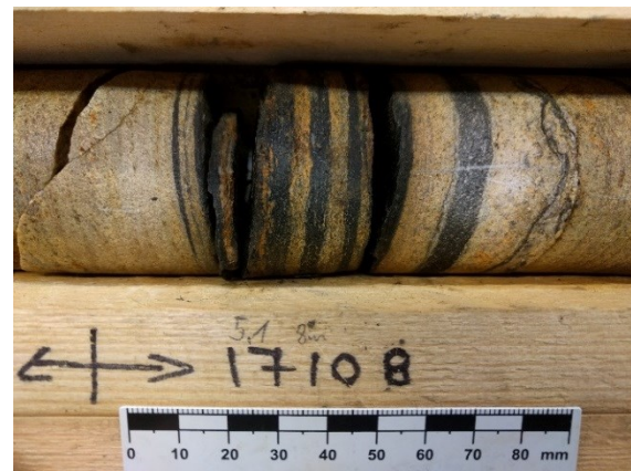
Fig. 15. Drill core showing 0.5-cm-thick parallel interlayers of mafic tuffites and arkose quartzites indicating a volcaniclastic sedimentation. Drill core MJ-5, depth 8 m.
