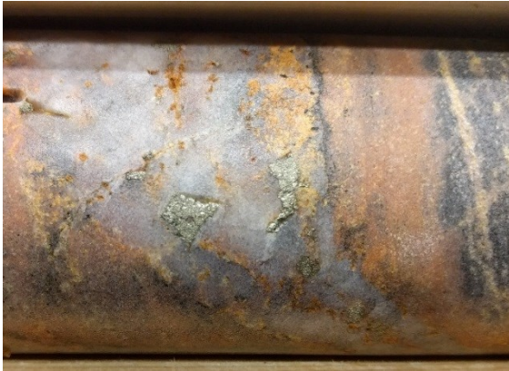
Fig. 71. Drill core showing a typical barren quartz-pyrite vein with proximal alteration zone. Drill core MJ-7, depth 30 m.
