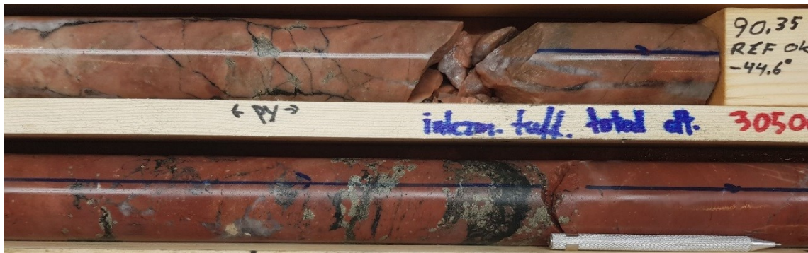
Fig. 57. Drill core showing tourmaline-rich pyrite mineralization in intensively silicified intermediate tuffite. The mineralization itself lacks quartz veining, but the silicification is very strong. Drill core 18MUS014, depth 90 m.
