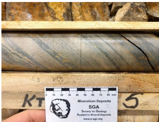
Fig. 14. Drill core showing least altered metasedimentary rock. The amount of mica is strongly varying in the rock package and changes gradually or sharply. Drill core MJ-5, depth 24.7 m.
