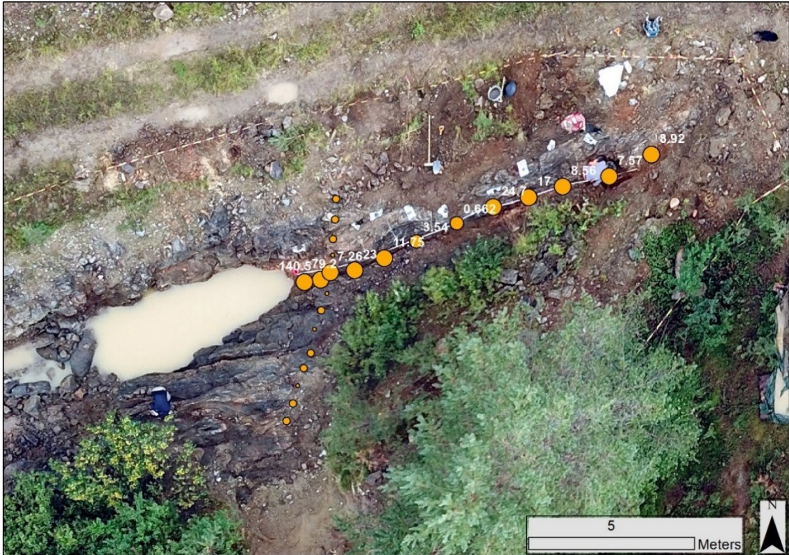
Fig. 104. Close up view of Fig. 103 (western part of trend 1) showing FireFox Gold channel samples with Au concentrations. The thickness and the gold grades of the outcropping main mineralized vein increase towards the left of the aerial photograph, indicating a pinch and swell structure of the mineralized veins.
