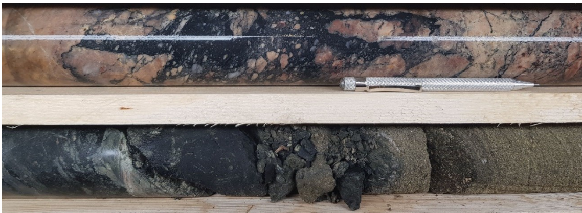
Fig. 69. Drill core showing a massive tourmaline vein brecciating a strongly albitized intermediate tuffite host rock (top row). In the center of the bottom row, massive tourmaline in totally altered mafic host rock (left), with a totally carbonated zone on the right. Drill core 18MUS013, depth 174 m.
