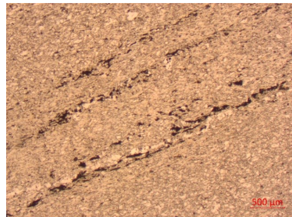
Fig. 25. Photomicrograph of intermediate tuffite. Muscovite rich layer associated with abundant hematite, also forming a foliation in the rock. Linear polarizers, field of view ~6 mm.
