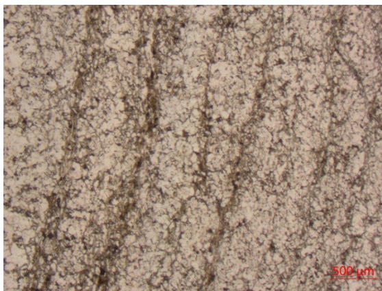
Fig. 24. Photomicrograph of intermediate tuffite. Thin biotite bands (brown) form a weak foliation in the rock. Linear polarizers; field of view ~6 mm.
