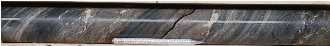
Fig. 21. Drill core showing least altered intermediate tuffite with biotite rich bands. Drill core 18MUS013, depth 184 m.
