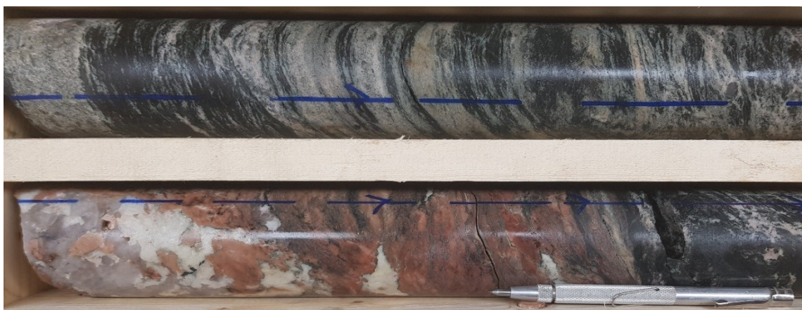
Fig. 58. Drill core showing a massive quartz-albite vein silicifying and albitizing the mafic tuff host rock. Drill core 18MUS013, depth 128 m.
