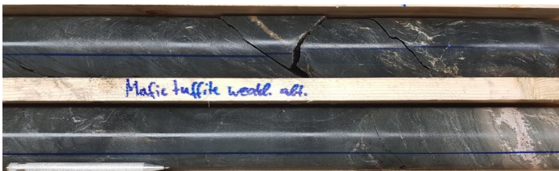
Fig. 27. Drill core showing least altered mafic tuffite. Drill core 18MUS013, depth 180 m.
