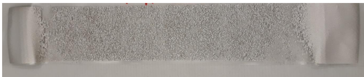
Fig. 35. Delaminated sample with manufacturer 2 paste.
