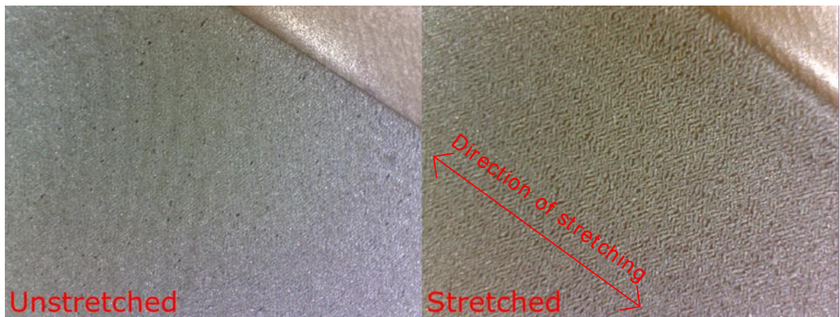
Fig. 38. Microscope image of full-filled sample at unstretched and 20 % stretched state.
