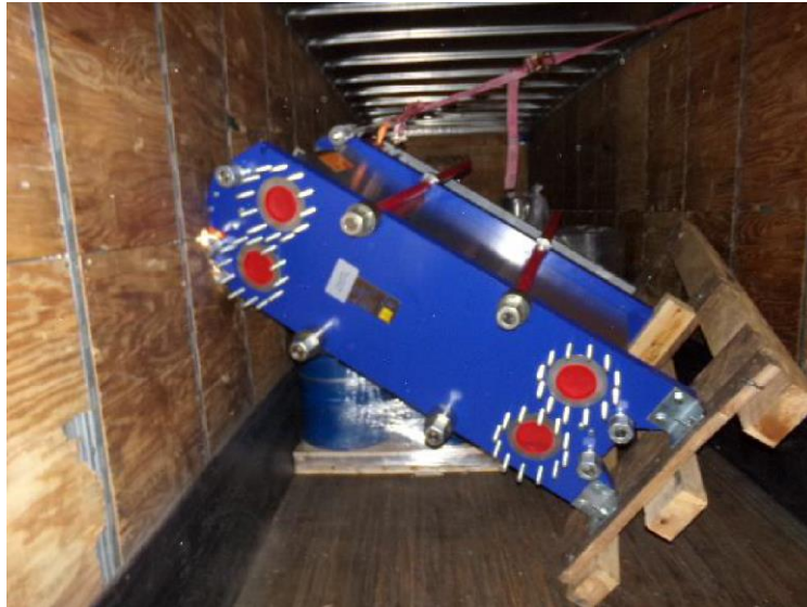
Figure 34. Product tipped over in the cargo container due ineffective securing
