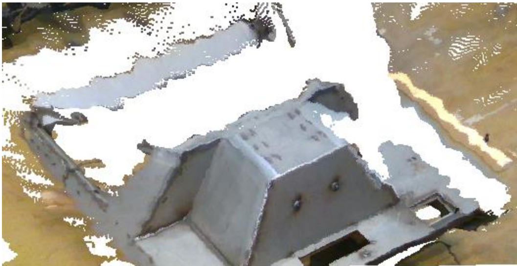
Figure 61. Colored 3D-depth image provided by the RealSense D415.
