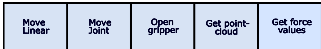
Figure 31. Example of different primitives in skill-based programming.
