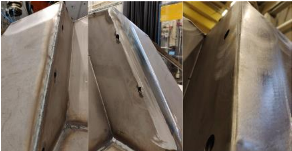
Figure 65. Seam in different phases from left to right: without grinding, after vertical grinding and after rounding movements.
