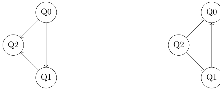
(a) Coupling map of original circuit of the for-loop of X gate. (b) Coupling map of adapted circuit of the for-loop of X gate.
