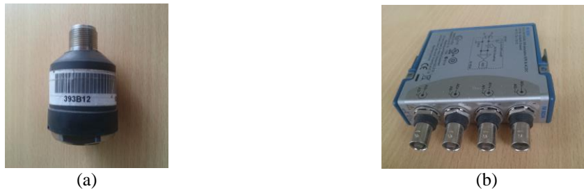
Figure 2. Acceleration monitoring equipment (a) PCB 393B12 - accelerometer sensor (b) cDAQ-9234 acquisition system.
