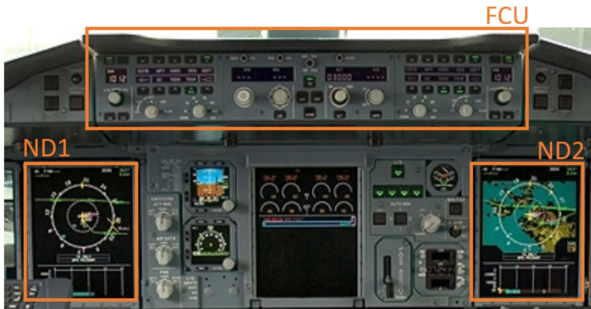
Fig. 4. The cockpit layout relevant to the proposed design
