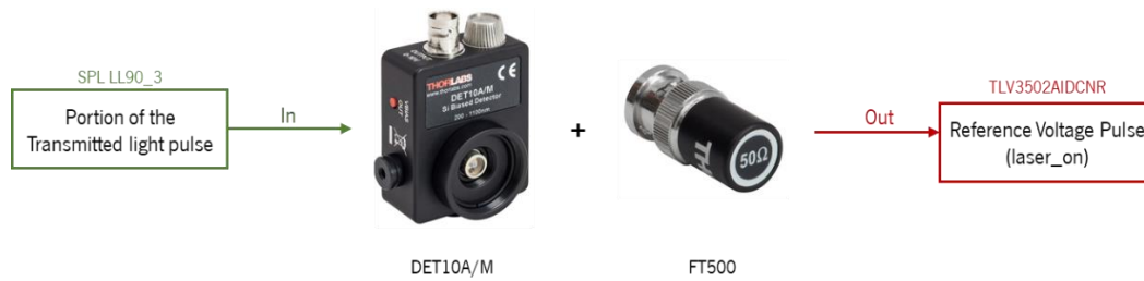
Figure 71. Simplified representation of the process for generating the reference voltage pulse.
