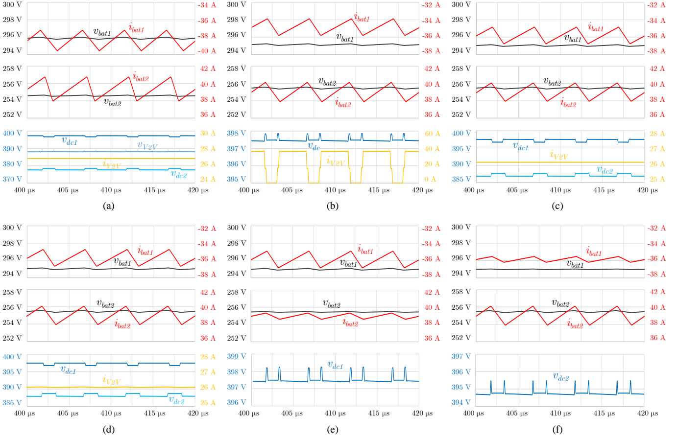
Fig. 4. Simulation results of the configurations for V2V power transfer between two EVs without using additional power converters: (a) ac-to-ac (A2A); (b) dc-to-dc (D2D); (c) dc-to-ac (D2A); (d) ac-to-dc (A2D); (e) ac-to-battery (A2B); (f) battery-to-ac (B2A).
