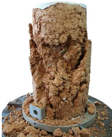
Figure 22. Typical failure mode of rammed earth cylinder
