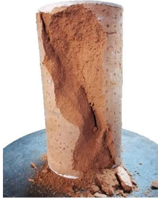
Figure 23. Typical failure mode of earth-based mortar
