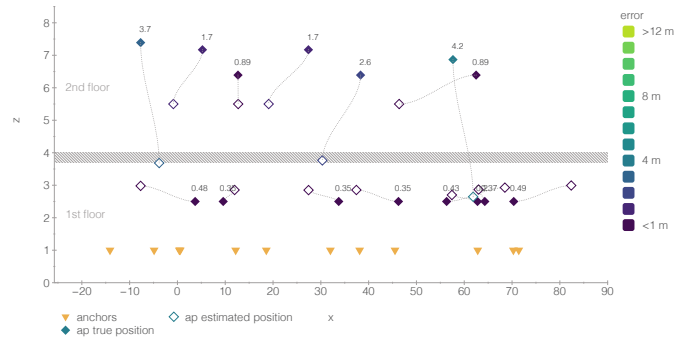
Fig. 6. APs Z Error DSI 1st and 2nd Floors
