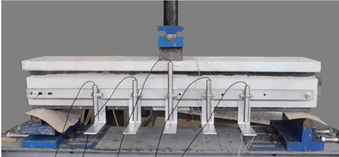
Figure 95 – Composite beam ready for testing [113].
