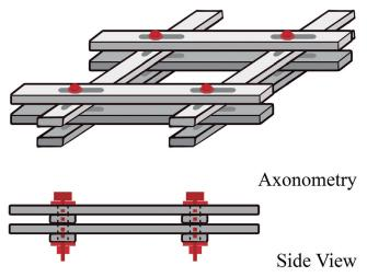
Figure 7. Double layer bolted connections
