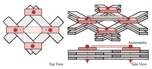
Figure 8. Diagonal locks with timber elements
