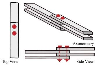
Figure 9. Bolted connections in the same line
