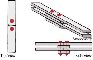
Figure 2. ZA Pavilion bolted connection
