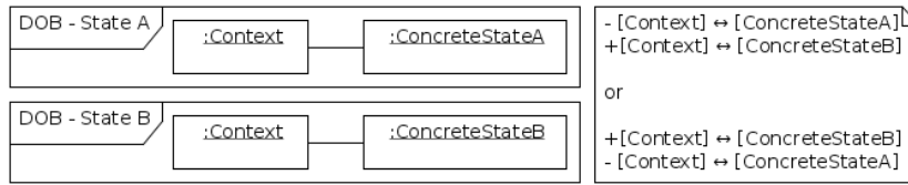
Fig. 2. Consider a UML Statechart organized through GoF’s State Pattern 6 with two states, ConcreteStateA and ConcreteStateB, and a transition from the first to the second one. Using UML object diagram it is just possible to express two detached diagrams each to a particular object’s configuration like in this example depicted as “DOB - State A” and “DOB - State B”. When applying the adaptive-graph approach, it becomes possible to model how can be the structural transition from configuration “DOB - State A” to “DOB - State B” (depicted in the “note”).
