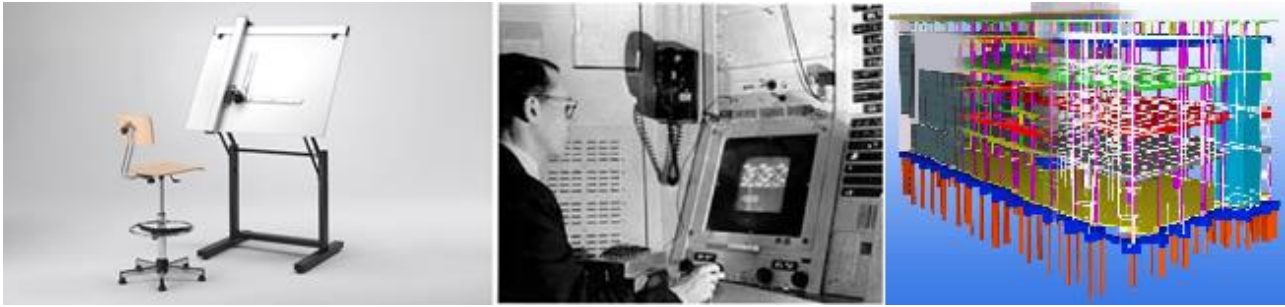
Figure 1: Left: Manual drafting table (Emmeitalia). Middle: Sketchpad (Sutherland, 1964). Right: BIM software (Tekla)
