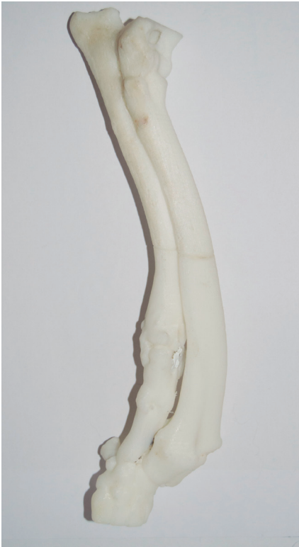
Fig.4. Printed 3D model in ABS, using a FDM printer, of the right forelimb antebraechium of the dog, lateral view.
