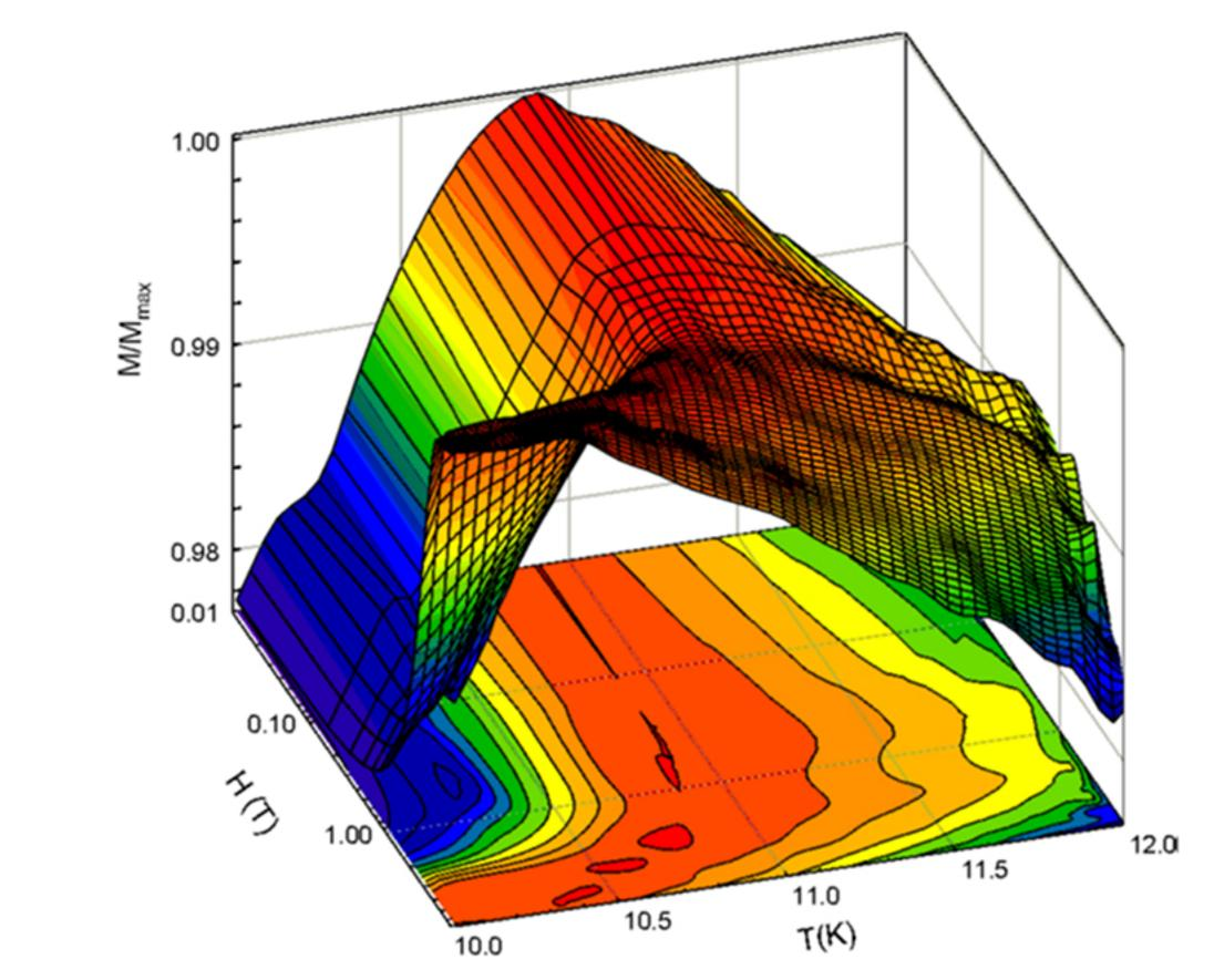
Normalized magnetization versus temperature and field for Ga Note the log scale on the H(T) axis. The critical temperature  $T_{r}$  at 11.2 K is just above the 10.9 K cusp at low fields. Above T, the spin-glass exhibits paramagnetism. Below the  $T_{c}$ , the magnetization exhibits behavior that suggests that a spin-glass transition is taking place.
