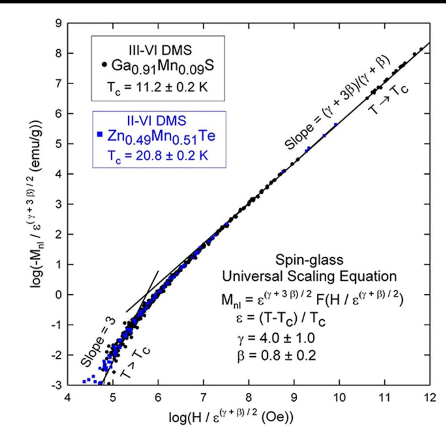
The nonlinear magnetization data analyzed according to a universal scaling model for  $Ga_{0.91}Mn_{0.09}Se$  and  $Zn_{0.49}Mn_{0.51}Te$ . There is an excellent overlap following the same universal scaling function over the entire range. The universal scaling relations was used to confirm Ga, Mn, Se along-Zn<sub>0.49</sub>Mn<sub>0.51</sub>Te undergoes a true spin-glass transition. side
