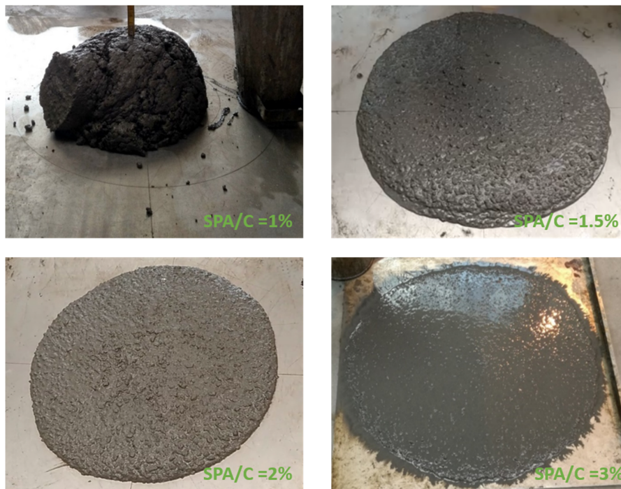
Figure 10. Detail of slump flow test.
