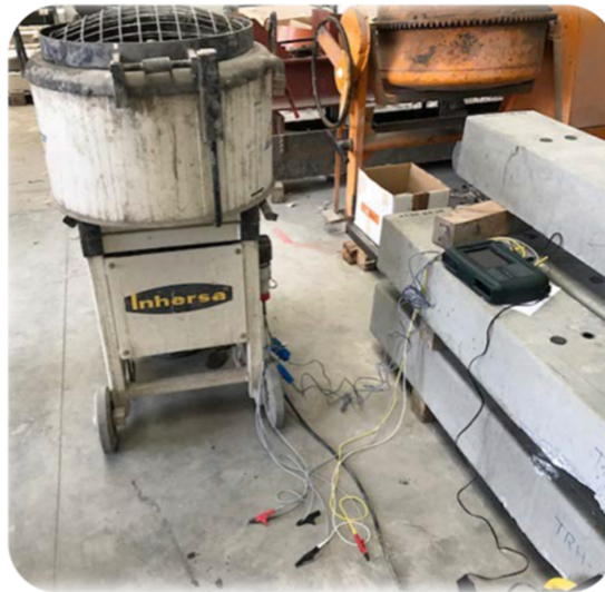
Figure 6. Instrument-fitted concrete mixer.
