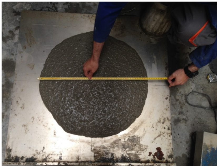
Figure 3. Slump flow test diameter measurement example.
