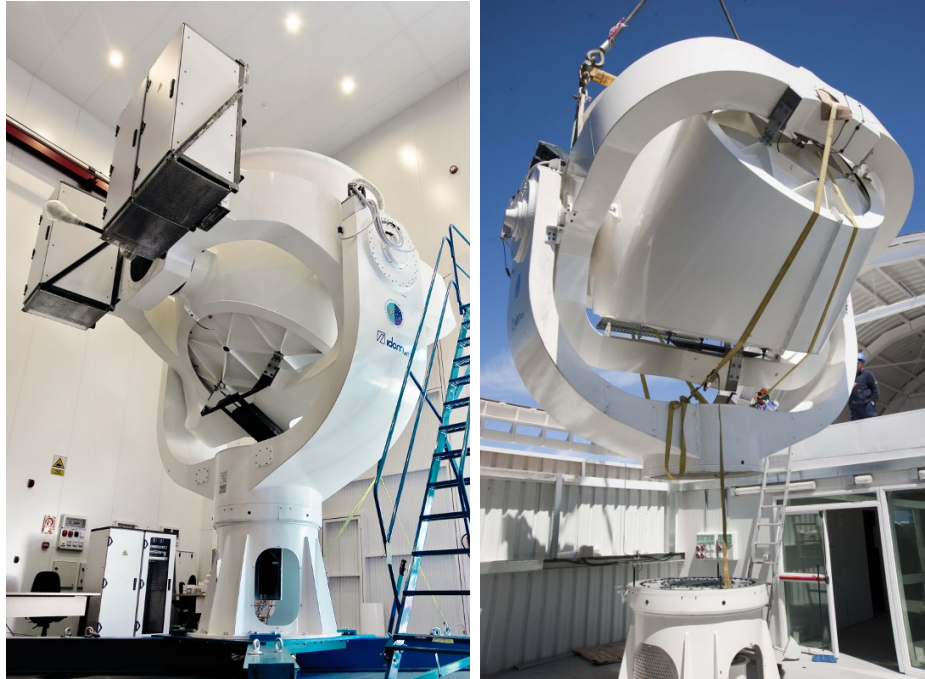
Figure 3. Left: QT1 at the IAC workshop (June 2009). Right: Installation of QT1 at the Teide Observatory (May 3rd, 2012).
