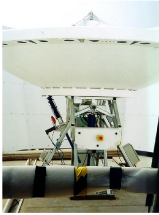
Figure 6. Left: One of the two antennas of the VSA source subtractor. This facility will be re-used to measure the polarisation of radio sources to correct the QUIJOTE-CMB 30 GHz maps. Right: Picture of the HWPs used for the VSA-SS.
