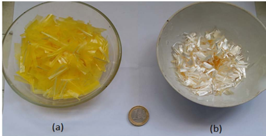
Fig.2. Types of synthetic fibers used in this work: (a) PO/A fibers and (b) PAN fibers.
