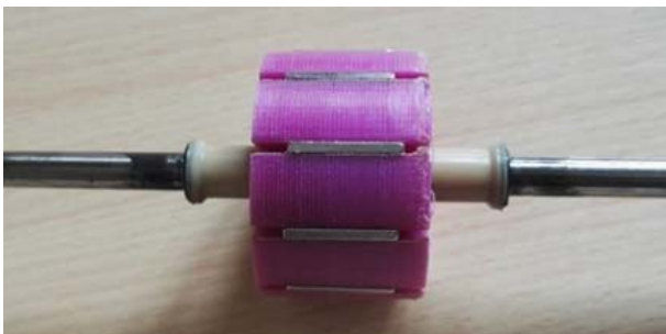
Fig. 7 Rotor with hard disk magnets.
