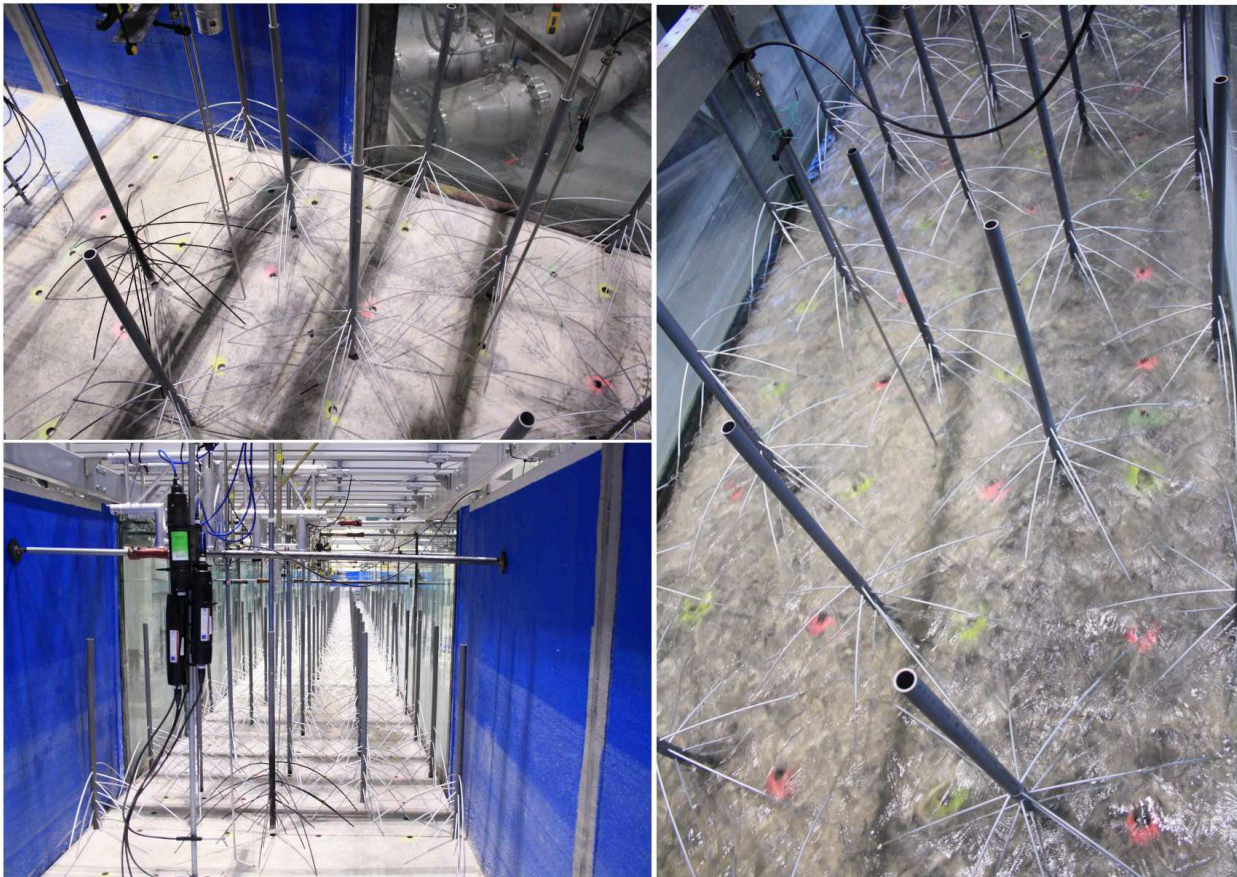
Fig. 1. Mangrove forest set-up. Views of the 26 m long forest with staggered configuration.
