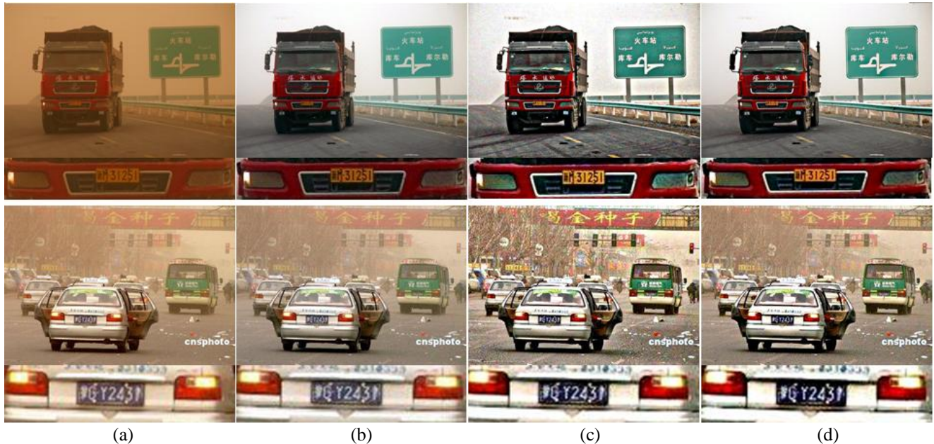
FIGURE 2. (a) Input sand-dust image and its license plate image. (b) Our white balancing enhanced sand-dust image and its license plate image. The remaining two images are the result of processing (b) using the methods of (c) guided Image filtering.[30] and (d) the proposed guided Image filtering.
