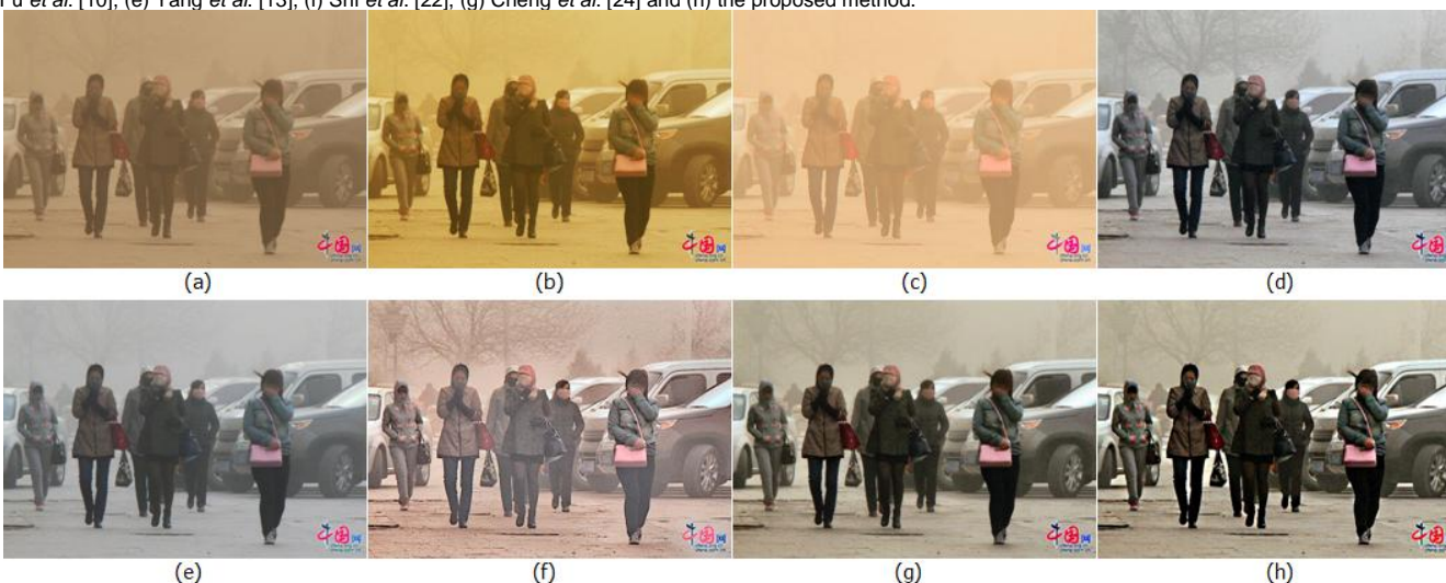
FIGURE 6. (a) Input sand-dust image. The remaining seven images are the restoration results generated by the methods of (b) Alameen [12], (c) Li et al. [4], (d) Fu et al. [10], (e) Yang et al. [13], (f) Shi et al. [22], (g) Cheng et al. [24] and (h) the proposed method.
