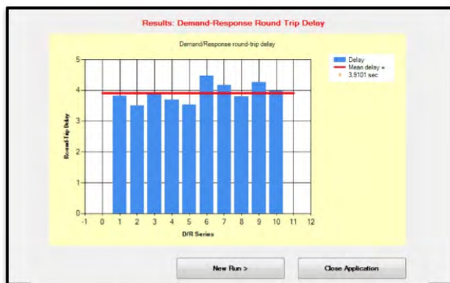
(b) Latency Graph of GUI Output
