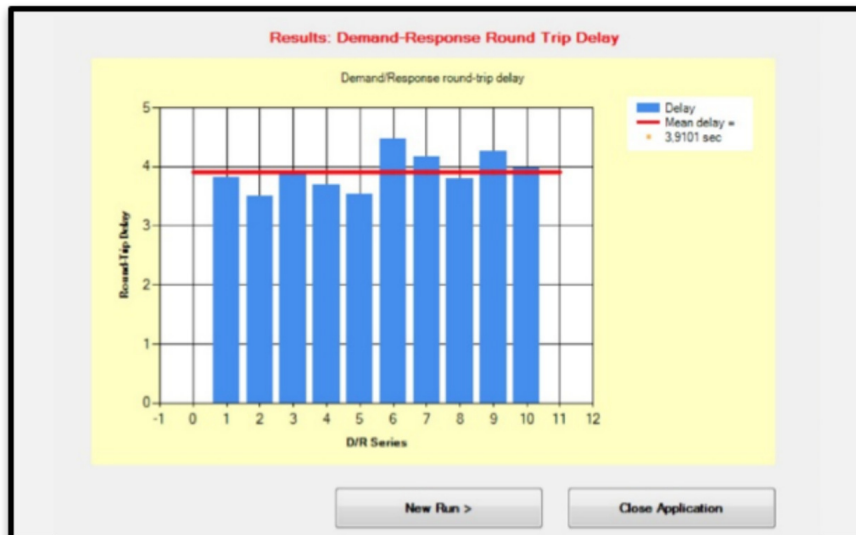
(b) Latency Graph of GUI Output
