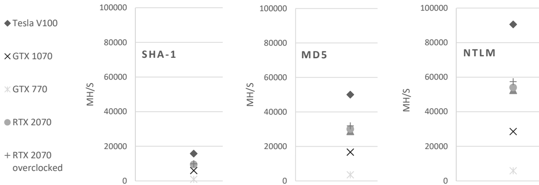
Figure 3: Performance of the three hashing algorithms on all GPUs listed in Table 2
