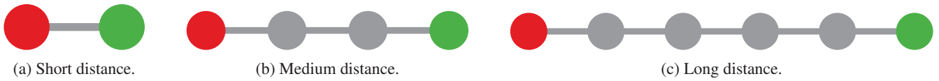
Figure 3: The expectation of the chain test. Origin node in red, destination node in green. As the chain gets longer, we expect the distance measure to return higher values.
