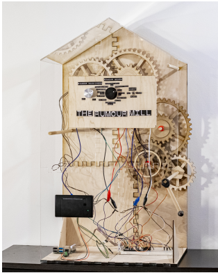
Figure 1: The Rumour Mill makes the process of creating rumours by means of NLP technology explicit for users by letting them interact with tangible controls that alters parameters for the AI-generated text.
