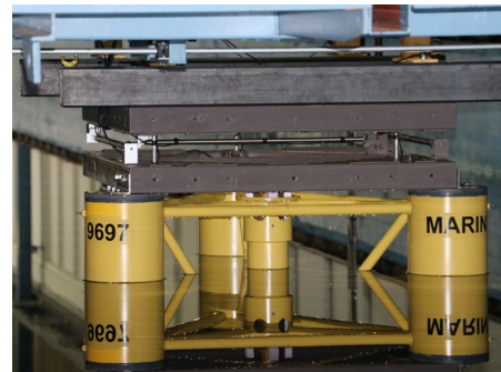
Figure 2: Configuration 2, OC6-DeepCwind floating semisubmersible attached to a carriage – seen from +x to -x (photo by Amy Robertson, NREL)
