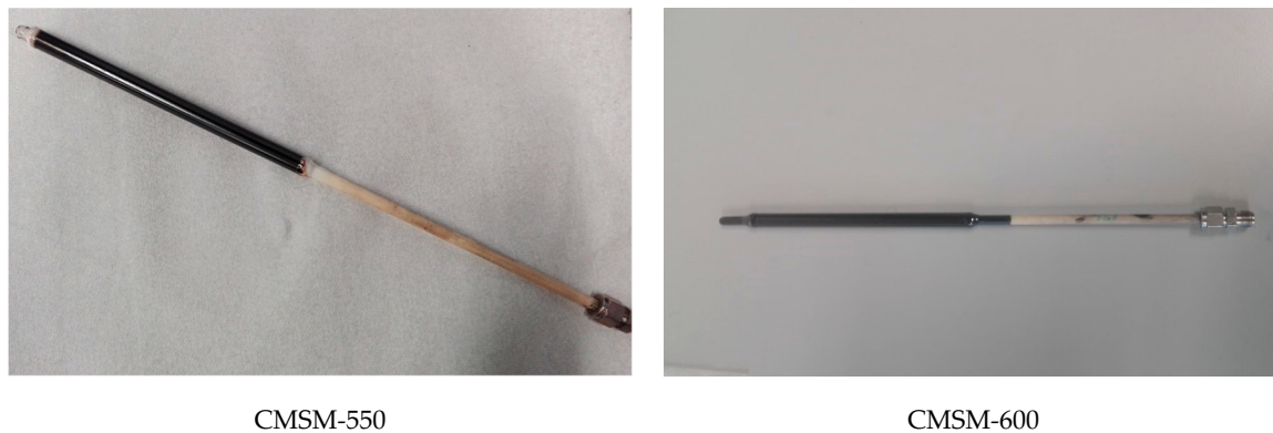
Figure 1. Pictures of the carbon molecular sieve membrane (CMSM)-550 and CMSM-600 carbonized at 550 and 600 °C respectively.
