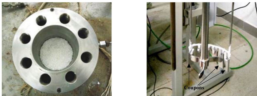
Figure 1. Autoclave filled with the lithium ternary molten salt (left) and detail of the rack with alloys specimens and the mixer (right).
