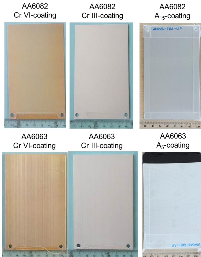
Figure 11. Representative photographs of AA6082 T6 (above) and AA6063 T6 (below) plates coated with Cr VI, Cr III and A coatings after 336 h of exposure to DHT.
