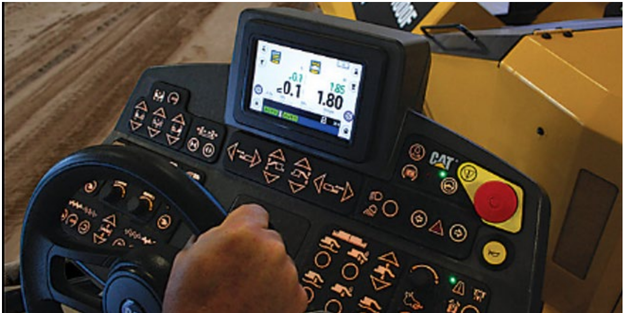
Figure 14. Example of Control Panel for Integrated Grade Control (Caterpillar)
