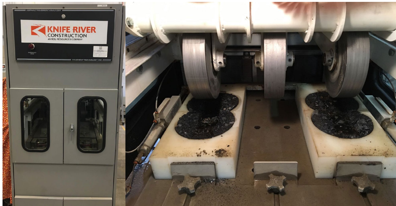
Figure 4. HWTT Equipment and Test Setup
