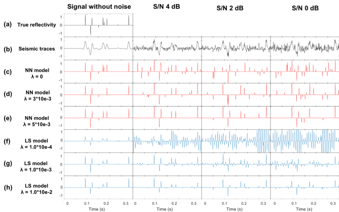
Figure 5.3. (a) True reflectivity, (b) Synthetic seismic traces computed from the true reflectivity using a simple convolutional model. White Gaussian noise is added with different S/N levels: noise-free, 4, 2, and 0 dB. Recovered reflectivity using neural network method with the L1 regularization parameter given by equation 5 of (c) \lambda = 0 , (d) \lambda = 3 \cdot 10^{-3} , (e) \lambda = 5 \cdot 10^{-3} . (f-h) Recovered reflectivity using least-squared method with the L1 regularization parameter (equation 7): (f) \lambda = 10^{-4} , (g) \lambda = 10^{-3} , (h) \lambda = 10^{-2} .
