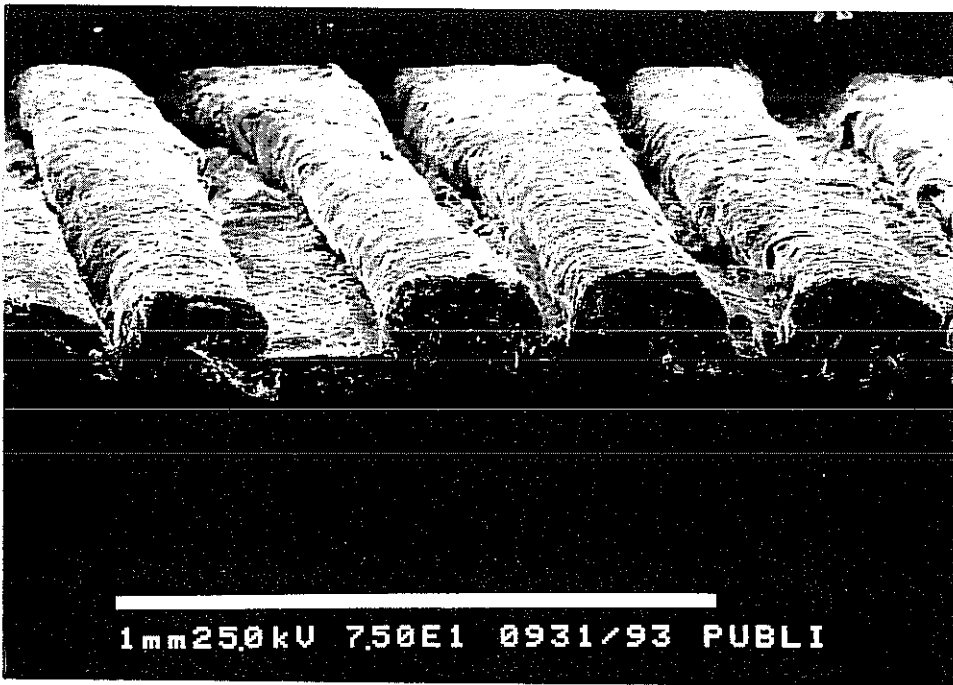
Fig. 7 Center Bursts and Crepe Wrinkles in Jumbo Rotogravure Reels
