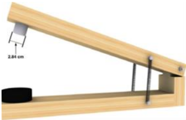
FIG. 2—Render of impact spatter rig. A 2.84-cm-diameter dowel was fitted to a wooden arm. Upon release the hammer-like arm strikes a modified hockey puck to generate an impact spatter. (Hakim & Liscio, 2015)
