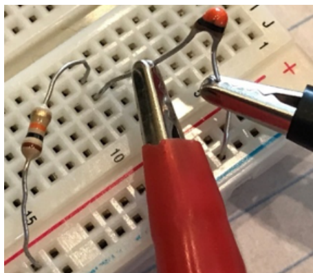
Figure 4.31. Photo of a Thermistor Voltage Divider: The thermistor is in series with a resistor, forming a voltage divider. Voltage is measured across the thermistor (see the red and black lead clips in the photo) to estimate temperature. Photo by Chad Davis.
