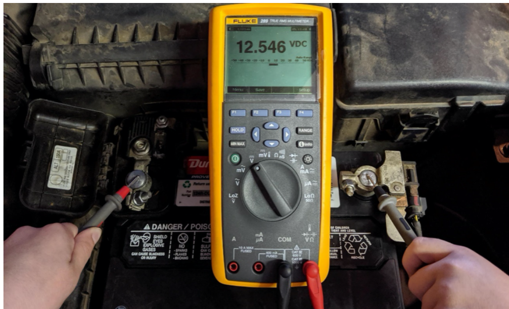
Figure 5.1. Car battery being measured with a multimeter: The red lead of the multimeter is placed on the positive terminal and the black lead is placed the negative terminal to read the battery voltage. Photo of battery measurement by Chad Davis.
