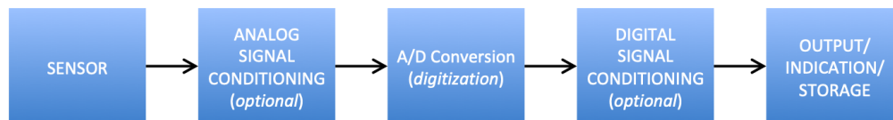
Figure 1.1. Analog and Digital Measuring Systems: The digital system also includes an analog-to-digital conversion block (called digitization in the diagram). The signal conditioning block is not present in some situations.
