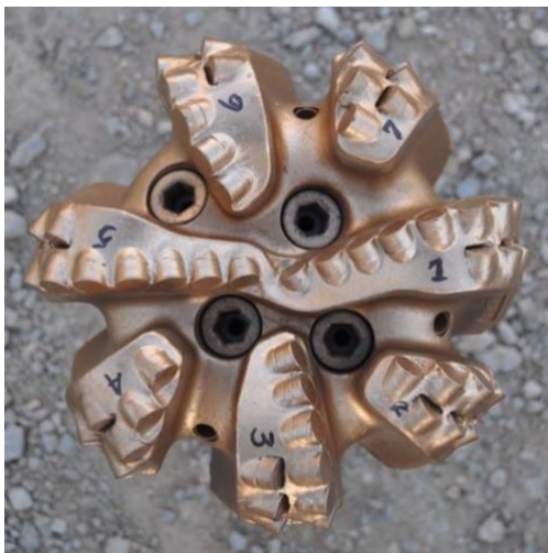
Figure 38: Bit #2 before drilling
