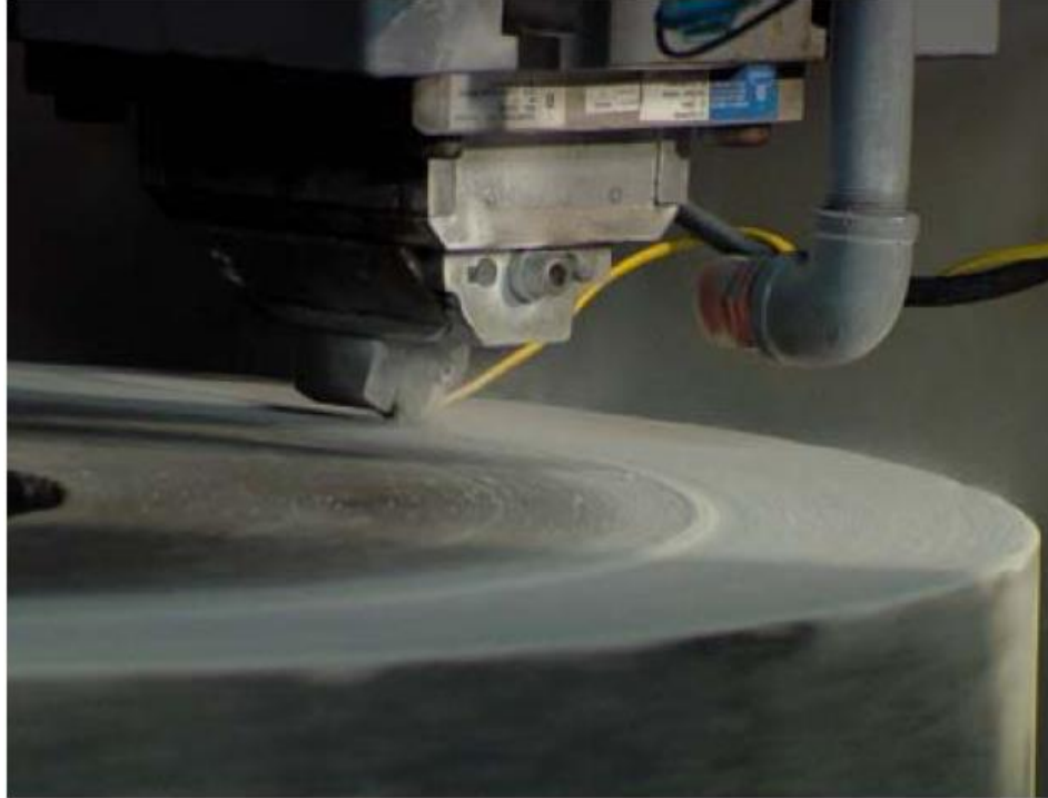
Figure 12: Single cutter dry testing
