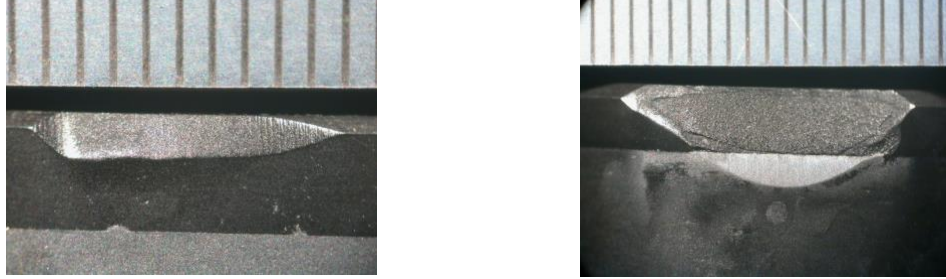
Figure 14: Cutter wear- PDC only (left) and Combined PDC and carbide (right)
