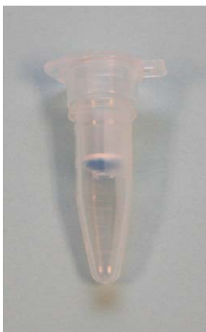
Figure 11. PrepFiler ® Lysep Column/hinge less tube assembly. Sample lysate is transferred from the Lysep column to the hinge less sample tube when the thin filter at the base of the column breaks upon centrifugation. The sample tube can then be separated and placed directly into the instrument.
