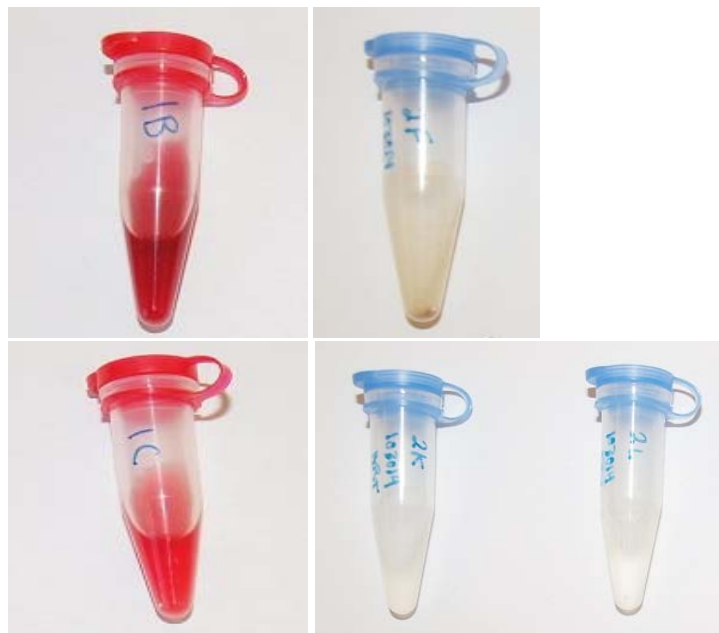
Figure 13. Comparison of physical appearance of control vs. bleach-treated samples. Control sample 1B (upper left)- 1:2 blood dilution vs. Sample 2F (upper right)- 1:2 blood mixed with neat bleach; Control sample 1C (lower left)- 1:10 blood dilution vs. Samples 2K and 2L (lower right)- 1:10 blood mixed with neat bleach and 1:10 blood mixed with 1:2 bleach, respectively.
