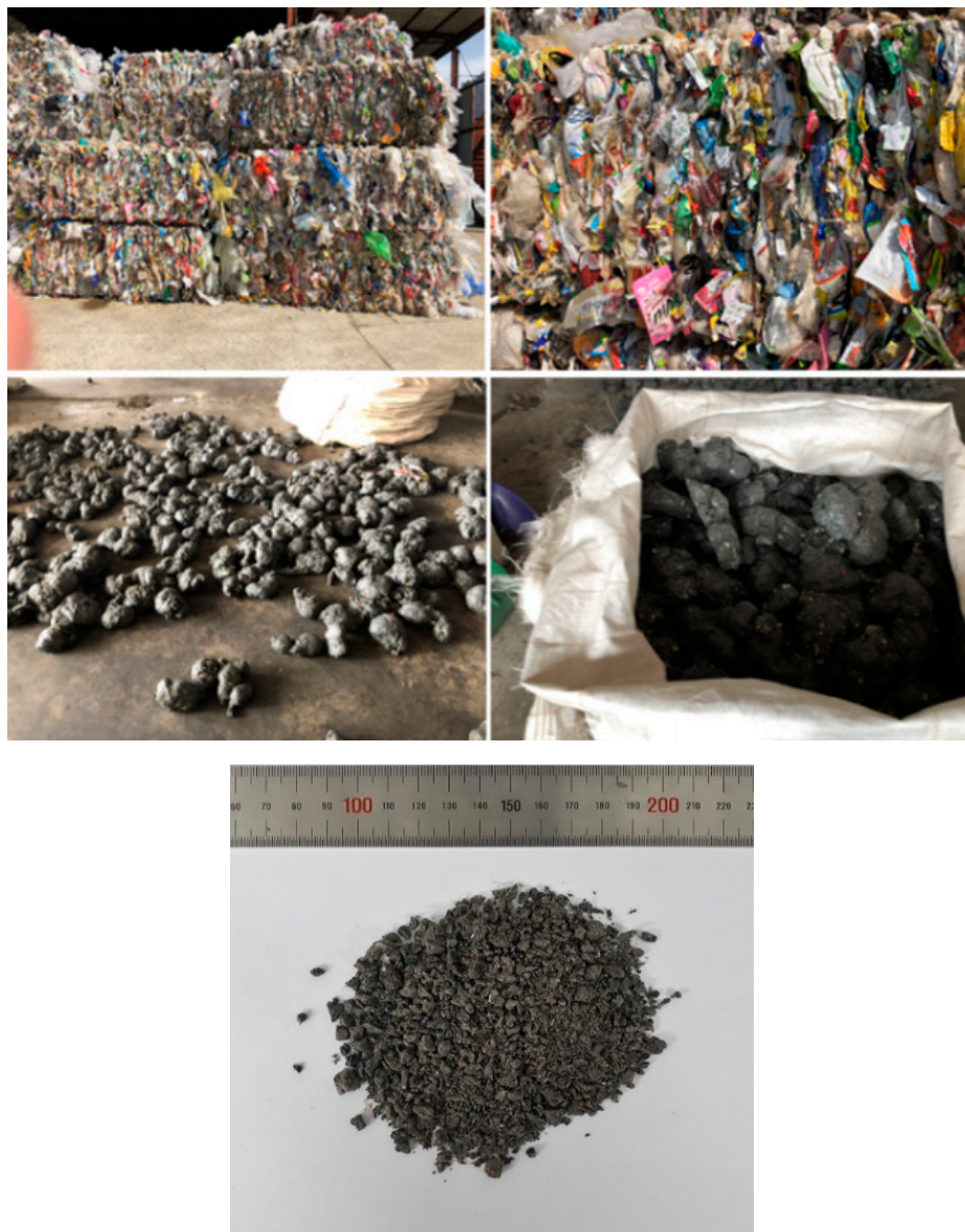
Figure 1. Recycling process of municipal plastic waste (MPW).
