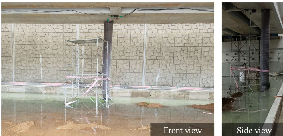
(b) Ring gauge measurement error due to a puddle
