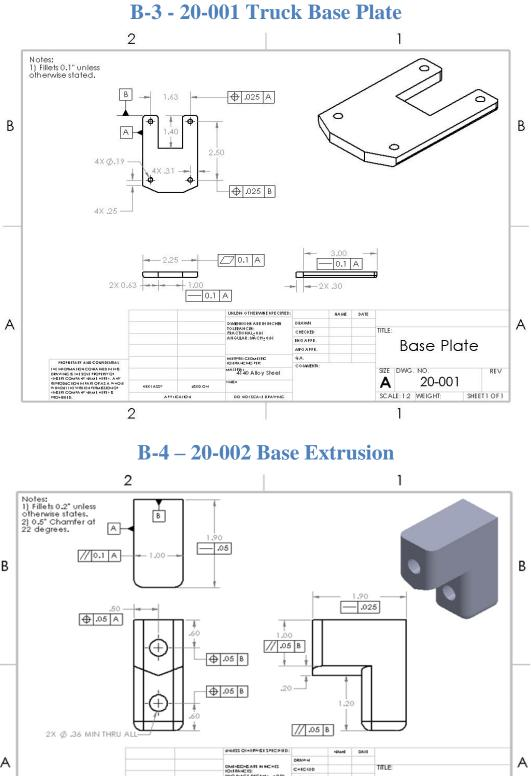
В A DMINEONE ARE NINCHES IOIEEANCES INO PLACE DECMAL 2006 INC APPR MC APPR **Base Extrusion** QA. CONNENIS SIZE DWG. NO. FORWARDE COFFAERS E PES 4140 Alloy Steel REV Α 20-004 -4151 A33 137804 SCALE: 1:1 WEIGHT: SHEET 1 OF 1 APPIRAIRS -----2 1
