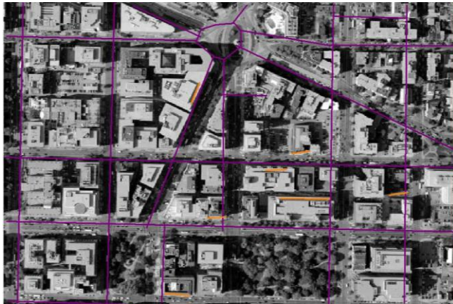
Figure 15. Vector map to be aligned (violet) and low quality automatic feature extract (ochre)
