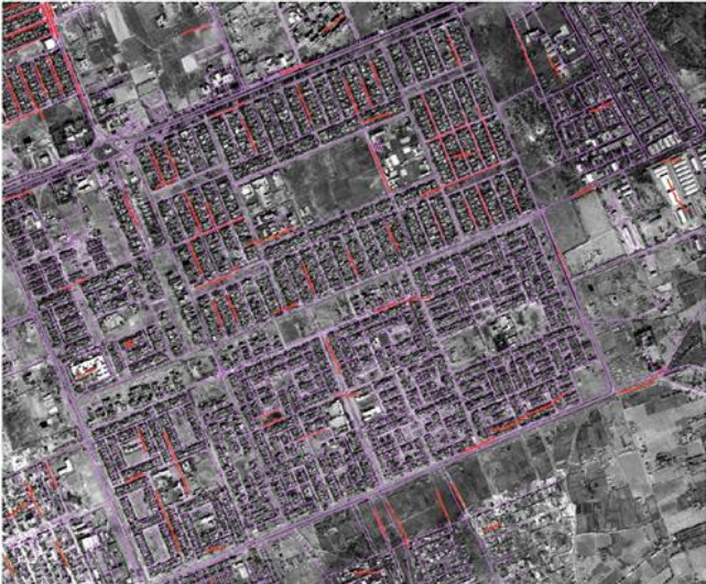
Figure 5. Extent of testing image (~ 3km × 3km) with automatically extracted roads (red)
