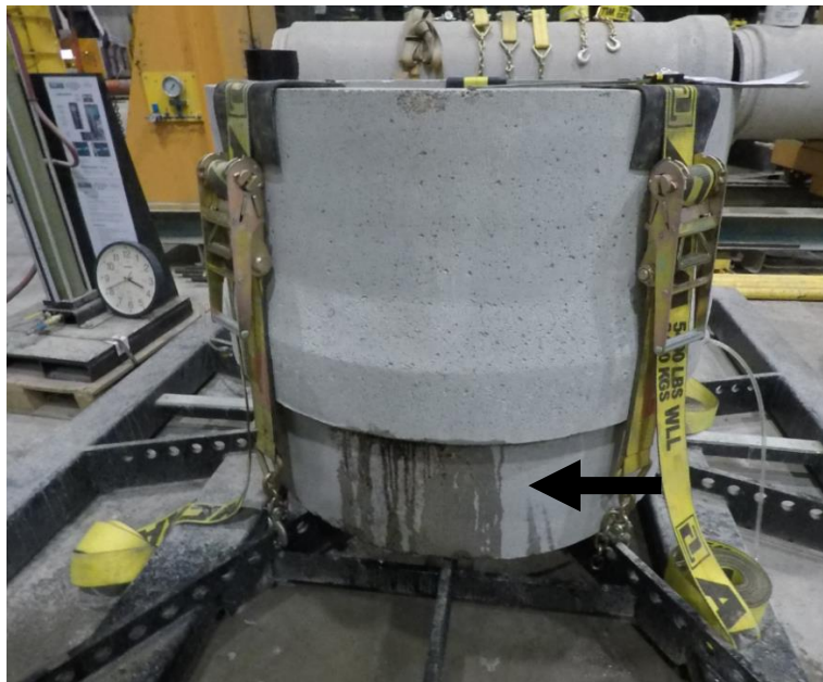
Figure 29: Leakage from Outside.
