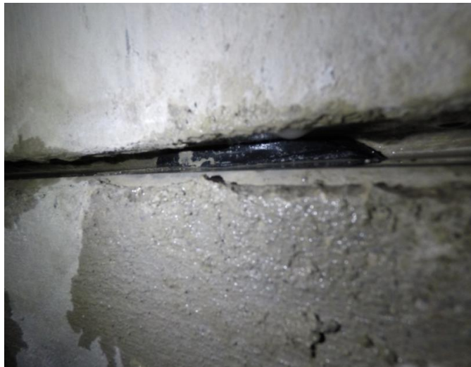
(a) Test #11 900 mm RCP, 475 kPa, Gasket Profile T02, 9 mm gap
