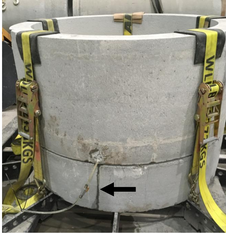
Figure 28: Minor External Leak During Test (1200 mm RCP, 375 kPa).
