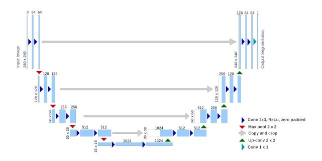
Figure 1.4: U-Net architecture used in the thesis. The model has been modified from the original to accept an input image size of  $240 \times 240$  pixel images and output a segmentation of the same size. Modified from Ronneberger et al. [35].
