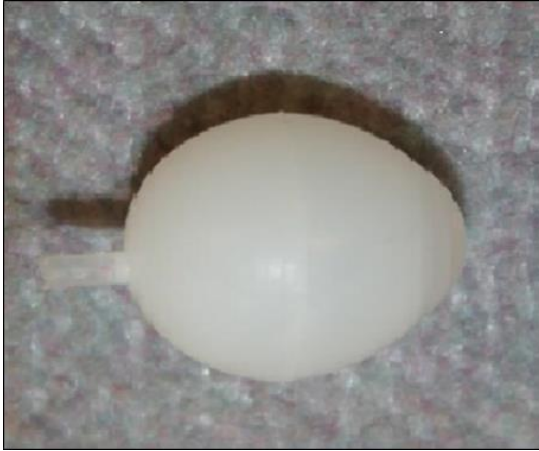
Figure 2.5: A tissue mimicking eye (PVA-C) at 6 freeze-thaw cycles modified from [34].
