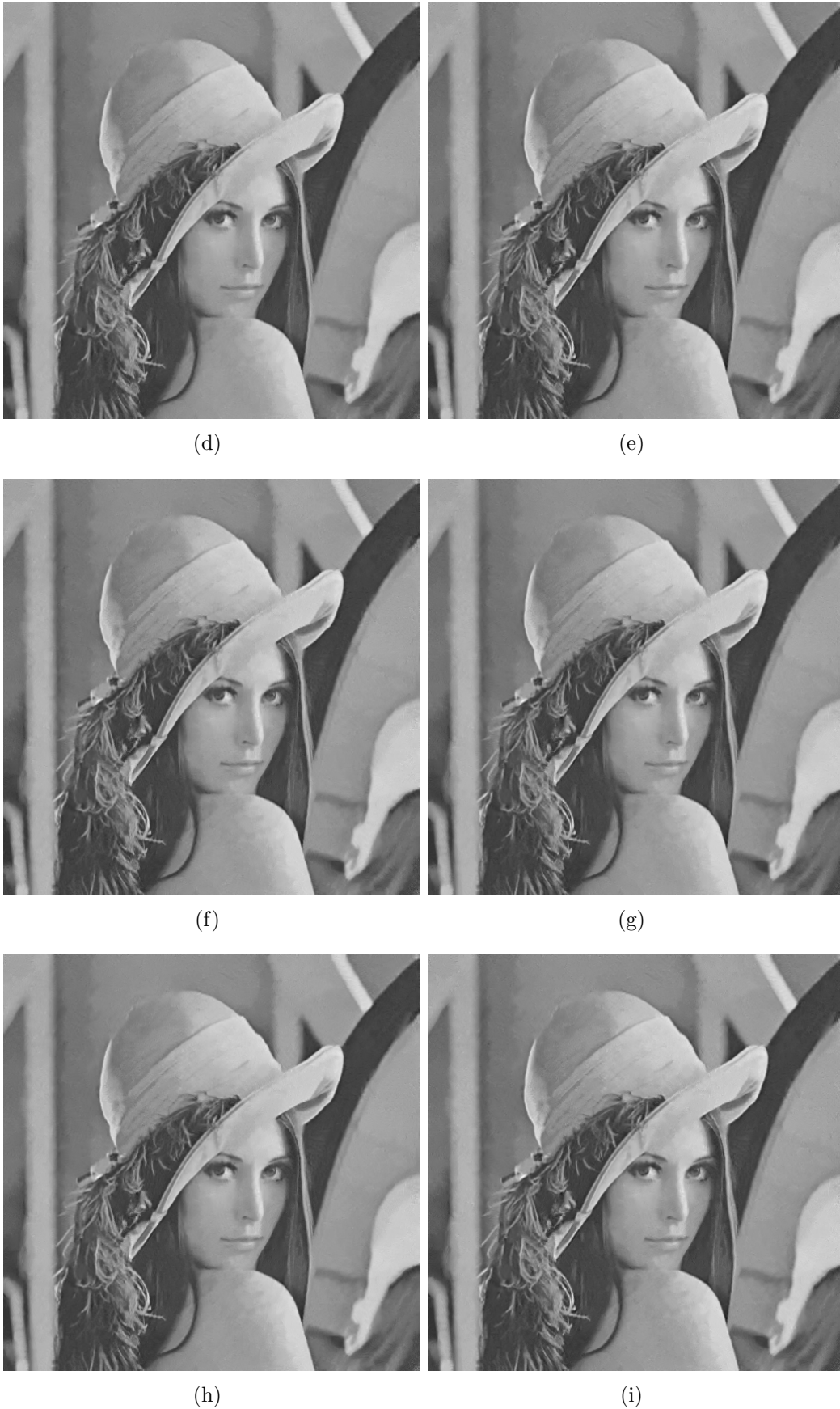
Figure 3.3: Lena image denoised by BM3D using different shaped kernels for stage one: (a) Original image. (b) Noisy image with \sigma = 20 (PSNR = 22.10). (c) Original BM3D stage one denoised image (PSNR = 32.30). (d) square kernel (PSNR = 32.19). (e) Circular kernel (PSNR = 32.12). (f) Horizontal kernel (PSNR = 32.16). (g) Vertical kernel (psnr = 32.15). (h) Diagonal with angle 135 kernel (PSNR = 32.20). (i) Diagonal with angle 45 kernel (PSNR = 32.16).
