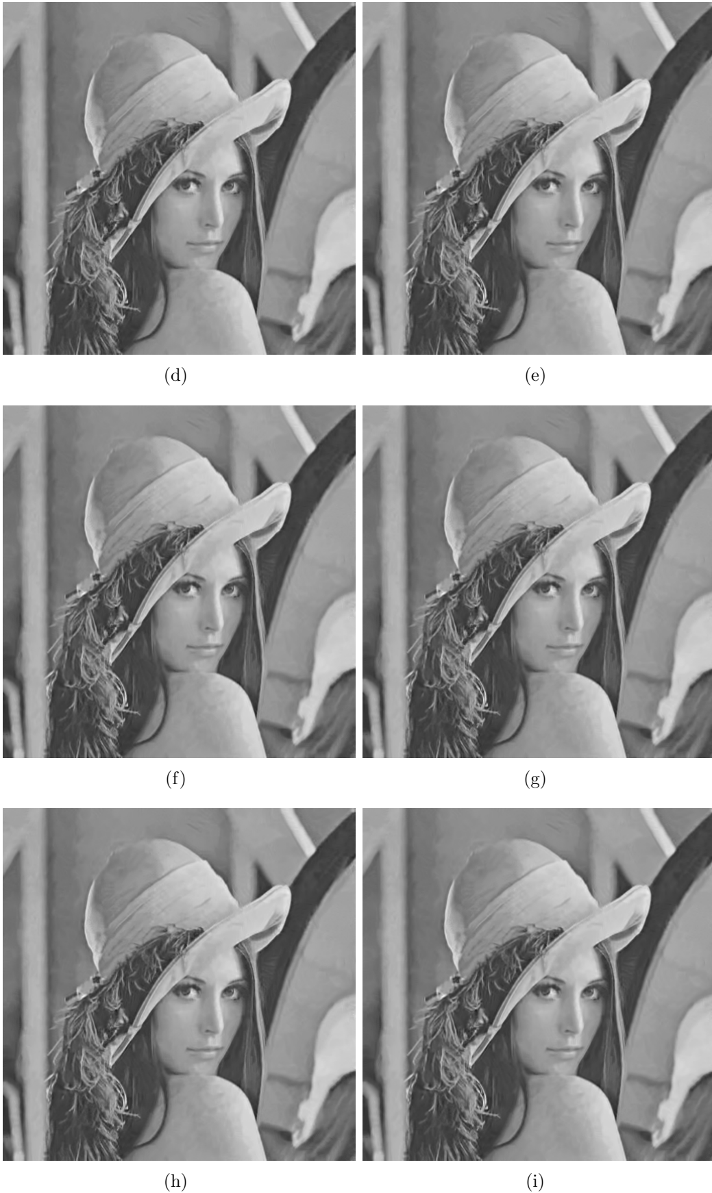
Figure 3.4: Lena image denoised by BM3D using different shaped kernels for stage two: (a) Original image. (b) Noisy image with \sigma = 20 (PSNR = 22.10). (c) Original BM3D stage two denoised image (PSNR = 32.83). (d) Square kernel (PSNR = 33.43). (e) Circular kernel (PSNR = 33.44). (f) Horizontal kernel (PSNR = 33.44). (g) Vertical kernel (PSNR = 33.42). (h) Diagonal with angle 135 kernel (PSNR = 33.44). (i) Diagonal with angle 45 kernel (PSNR = 33.45).
