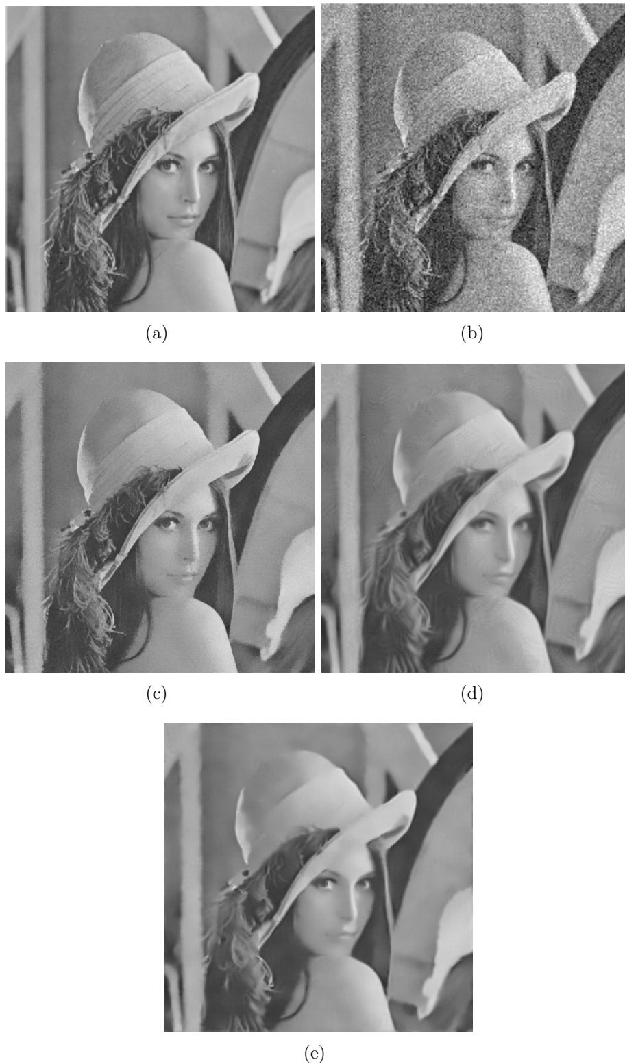
Figure 2.7: Lena Denoising using non-local means (nlm), statistical nearest neighbour (SNN), and fast shape adaptive non-local means (SA-Fast-NLM) approaches at \sigma = 20 . (a) Original image. (b) Noisy image (PSNR = 22.10 db). (c) Denoised using NLM (PSNR = 31.18 db). (d) Denoised image using SNN (PSNR = 31.22 db). (e) Denoised using SA-Fast-NLM (PSNR = 31.53 db)
