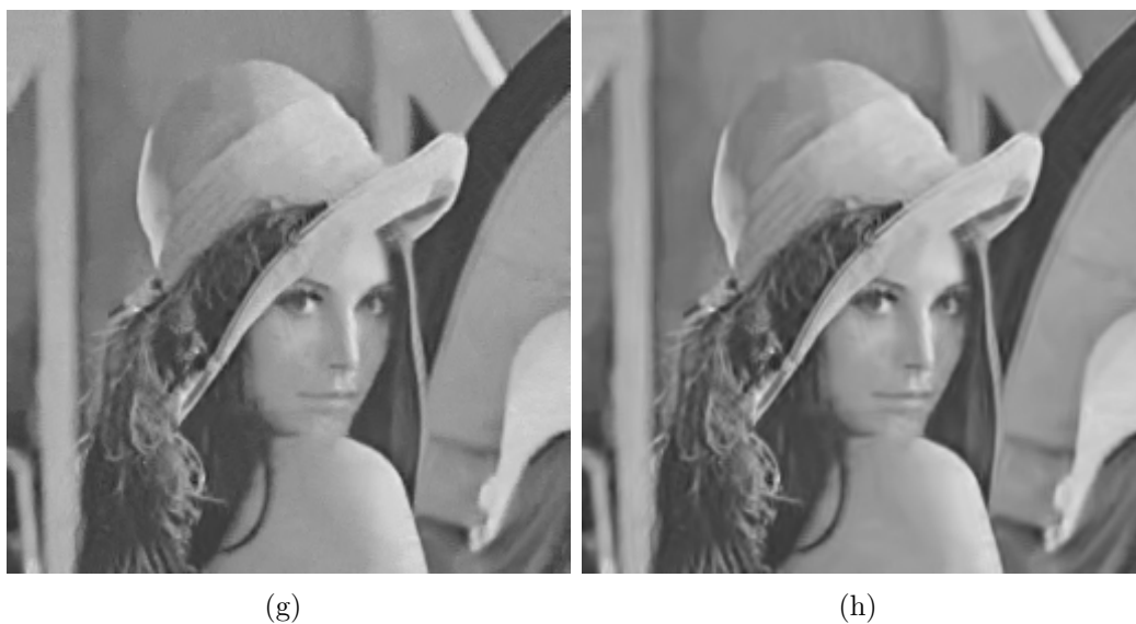
Figure 3.11: Denoised Lena image results using the proposed framework. (a) Original image. (b) Noisy image with \sigma = 20 (PSNR = 22.14). (c) Original BM3D after stage one. (PSNR = 32.23) (d) Original BM3D after stage two (PSNR = 33.77). Pixel based results, (e) Proposed framework after stage one (PSNR = 33.69). (f) Proposed framework after stage two (PSNR = 33.99). Patch based results, (g) Proposed framework after stage one (PSNR = 32.74). (h) Proposed framework after stage two (PSNR = 33.26)
