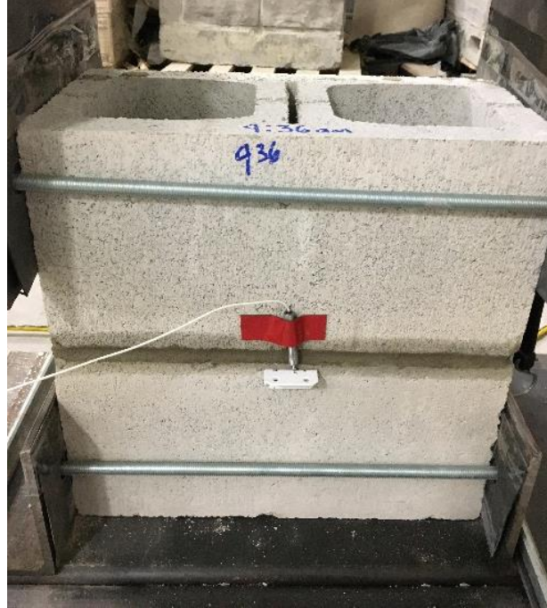
Figure 2.7: Attachment of LVDTs to a two-course masonry prism.
