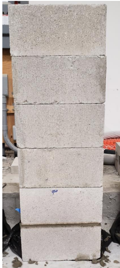
Figure 2.5: Finalized construction of a masonry assemblage for testing.
