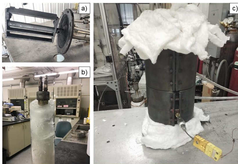
Figure 2.2 – Unit components; a) stirrer; b) condenser after pyrolysis; c) reactor;
