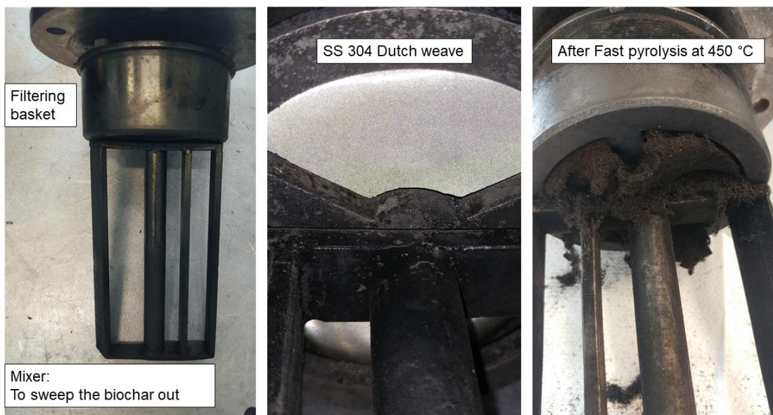
Figure 5.3 – Reactor filtering basket
