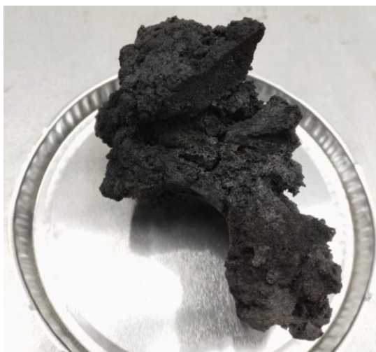
Figure 4.7 – Biochar produced at 500°C, 5°C min -1 from the sample with 60% lignin content
