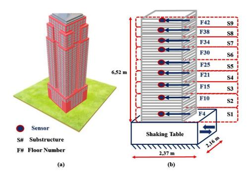
Figure 2.9: a) 3D model of the Hong-Kong 42 story High-rise Building. b) Scaled Prototype of the Substructures and Location of Sensors along with the Height of the Building.
