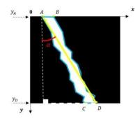
Figure 3.12: Calculation of Angle of Orientation of Crack.
