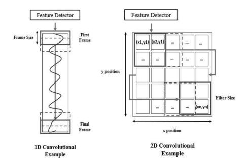
Figure 4.2: Difference between 1D CNN and 2D CNN.
