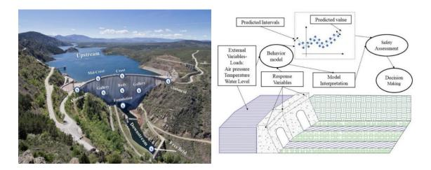
Figure 2.10: a) A disposition of the Installed Sensors in a Dam. b) Flow Diagram of DM Data Analysis.
