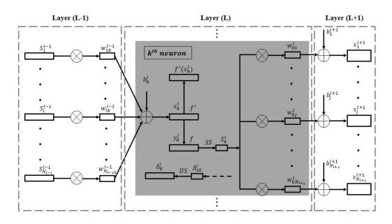
Figure 4.4: Three 1D CNN Consecutive Hidden CNN Layers. (reproduced and modified from Abdeljaber et al., 2017)
