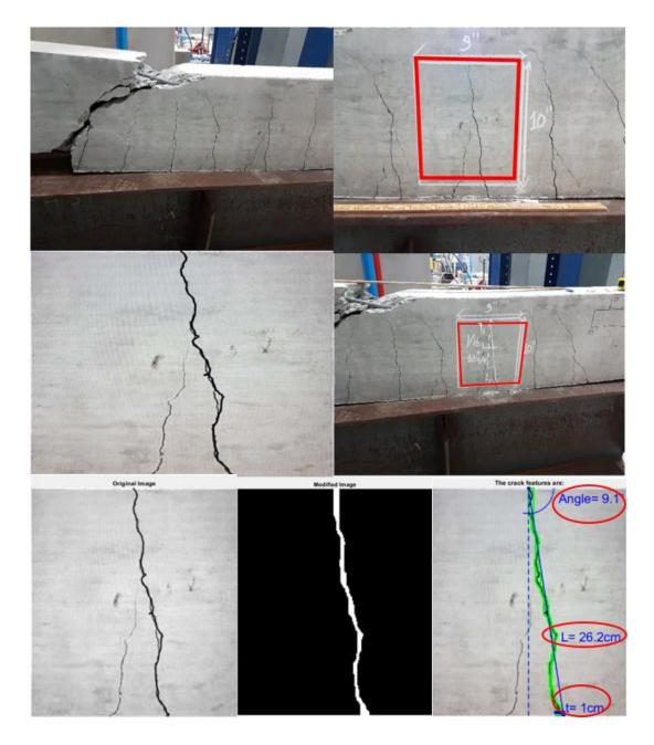
Figure 3.19: Calculation of Crack Features of the Damaged Beam under the Effect of Flexural Stress.
