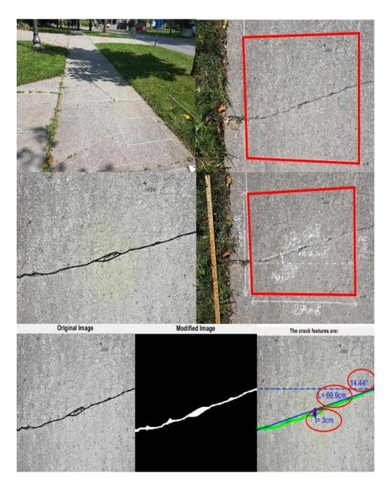
Figure 3.20: Calculation of Crack Features of Damaged Pavement under the Effect of uplifting of Tree Roots.
