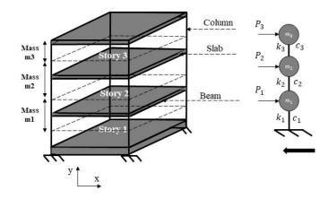
Figure 4.7: Three-Dimensional Model of a Three DOF System.
