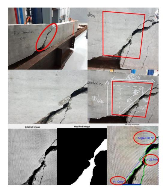
Figure 3.18: Calculation of Crack Features of the Damaged Beam under the effect of Shear Stress.
