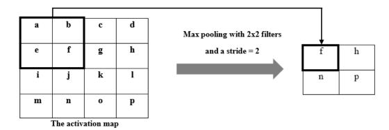
Figure 3.5: Pooling Operation.
