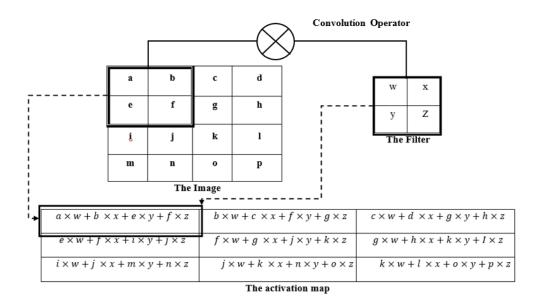
Figure 3.4: Convolution Operation.
