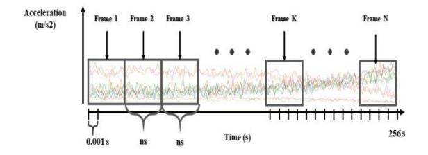
Figure 4.6: Example of a Signal Decomposition into N Number of Frames.
