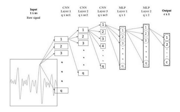
Figure 4.3: Example of 1D CNN Configuration with 3 CNN and 2 MLP Layers. (reproduced and modified from Kiranyaz et al., 2019)
