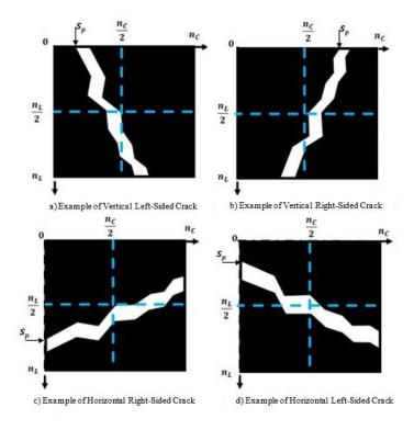
Figure 3.2: Example of Labeled Images According to the Proposed Method.
