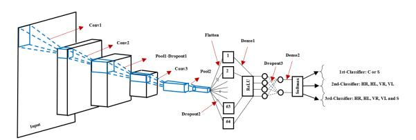
Figure 3.3: Overall Architecture of the CNN Classifier.
