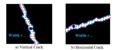
Figure 3.10: Width Calculation of the Crack.
