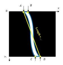
Figure 3.9: Length Calculation of the Crack.
