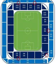
Figure 2.12: Sensors Installed in Giuseppe Mazzei Stadium, Italy.
