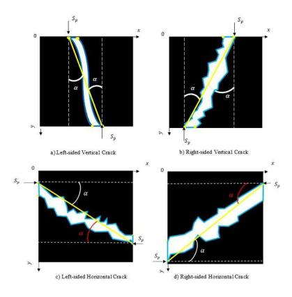
Figure 3.11: Configuration of the Angle of Orientation in the Image.
