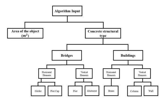
Figure 3.15: Database Inputs Model Incorporation.
